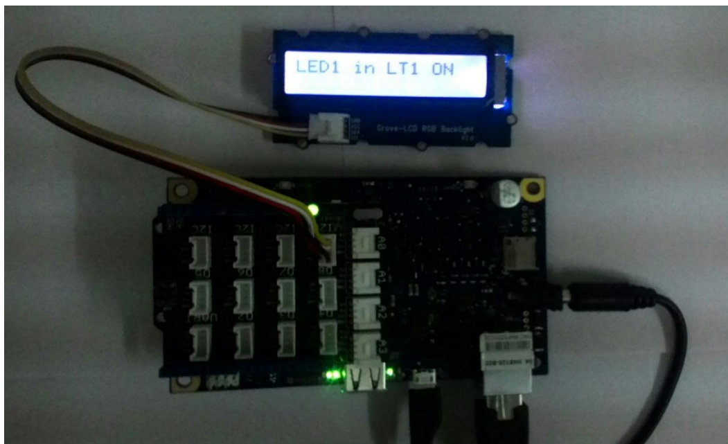
Figure 27: LCD displaying LED1 status when LED1 switch is pressed ON
