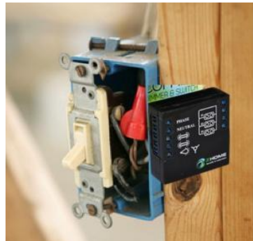
Figure 5: Z HOME Retrofit Solution
