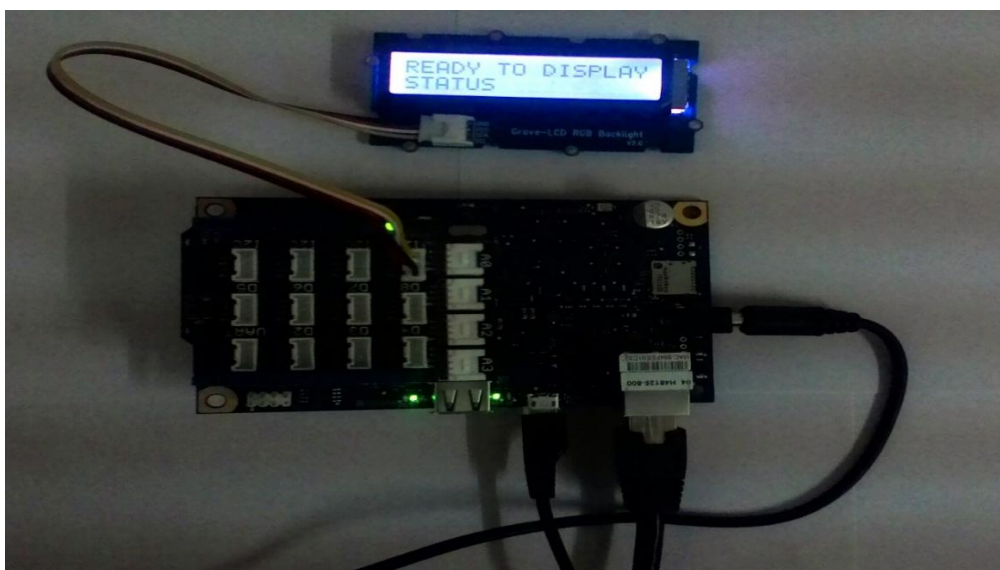
Figure 25: Circuit having LCD component connected to Server through Galileo
