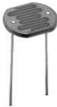
Figure 10: ORP12 Cadmium Sulphide photoconductive cell
