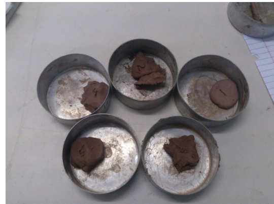
Some samples from liquid limit testing
