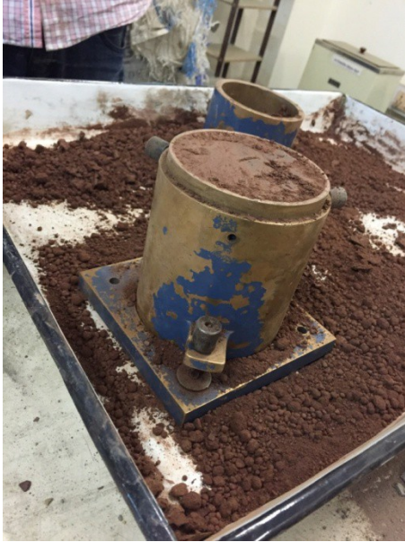
Proctor Compaction Test
