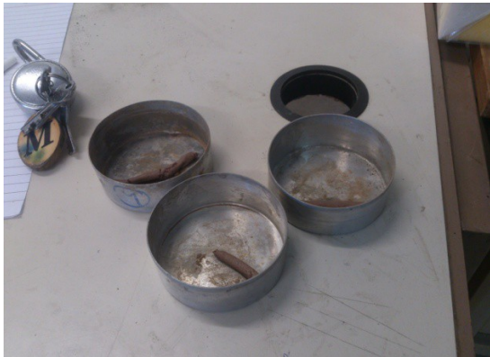
Some samples from plastic limit testing
