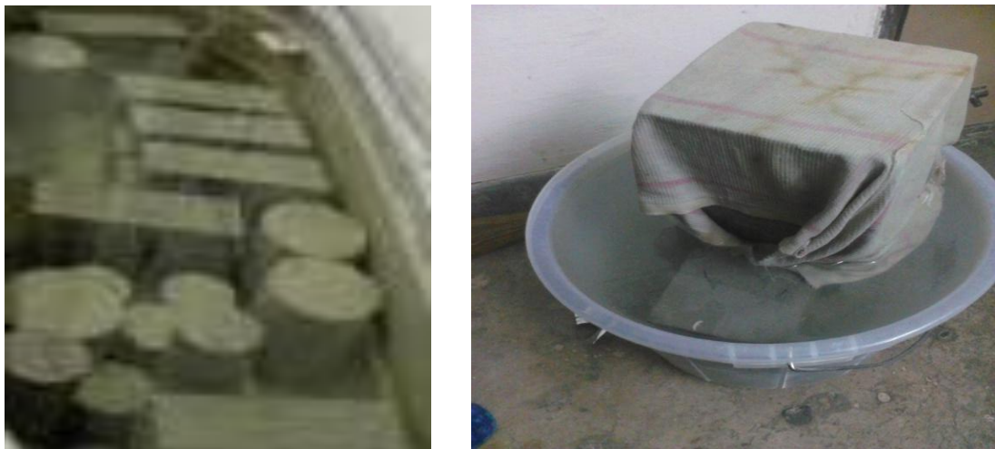
Fig 2: Curing of Immersion and Wet Covering Methods
