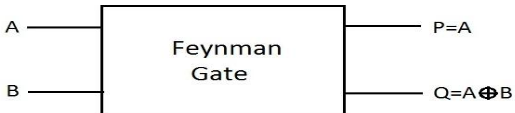
Figure 2.1: Block Diagram of Feynman Gate
