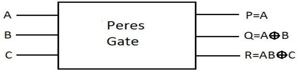
Figure 2.10: Block Diagram of Peres Gate
