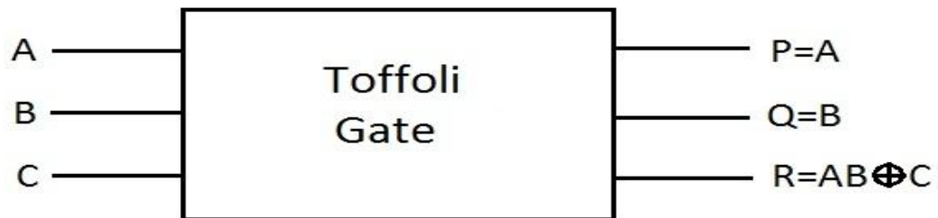
Figure 2.4: Block Diagram of Toffoli Gate
