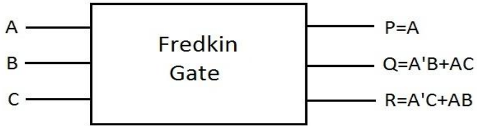
Figure 2.7: Block Diagram of Fredkin Gate
