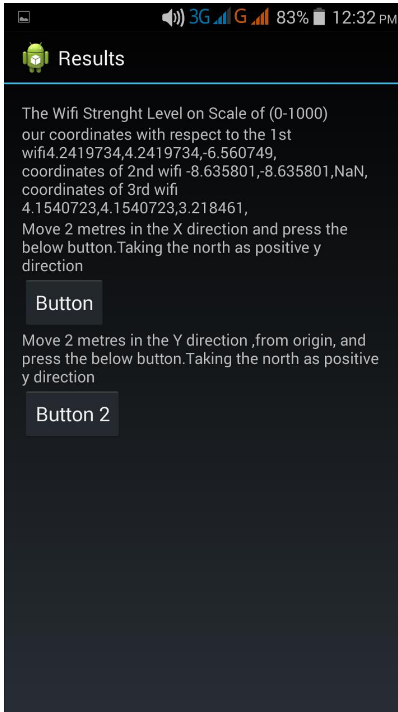
Figure 15. After going 2 meters in the x direction and clicking the first button and then going 2 meters in the y direction will give us 3 equations from which we can calculate 3 coordinates using the basic distance formula. We have assumed the coordinates of the user as zero zero in the beginning.
