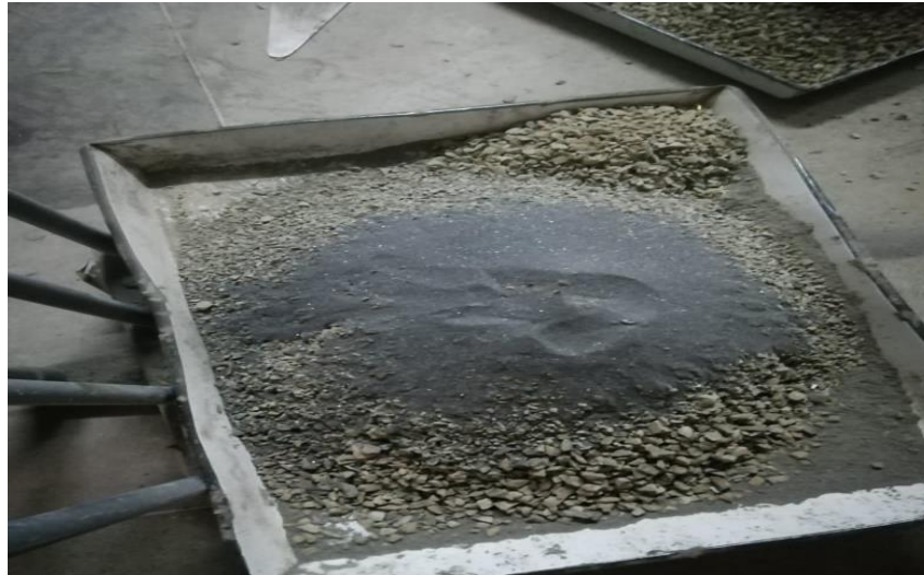
Fig 3.8 Addition of waste foundry sand in concrete mix
