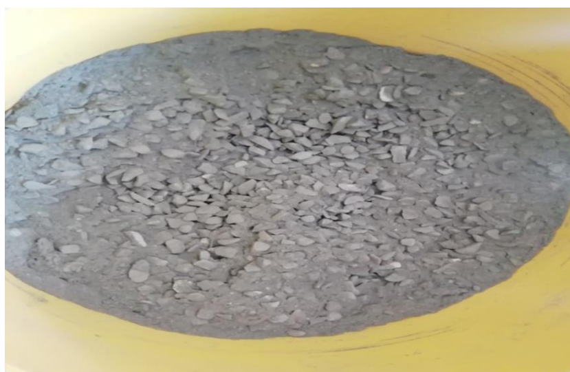
Fig 3.9 Dry mix of concrete mix
