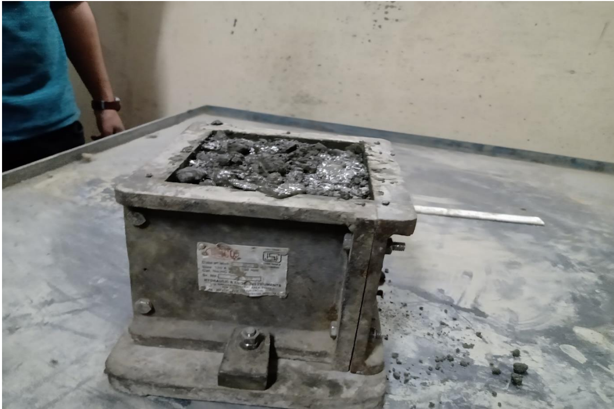
Fig 3.13 Casting of Cube
