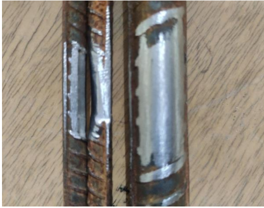
Figure 3.11: Rebar specimen prepared For bonding
