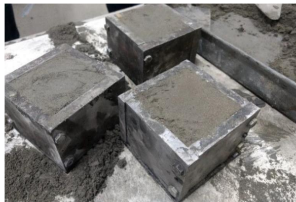
Figure 3.10: Cubes preparation for compression test
