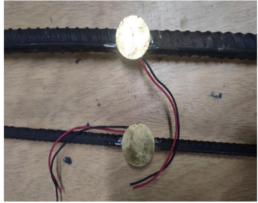
Figure 3.12: PZT on surface of rebars
