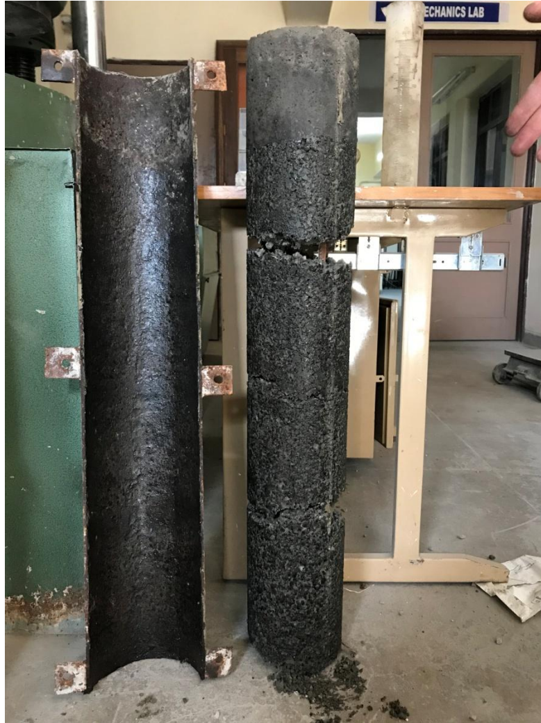
Figure 4.6 Failure due to improper compaction
