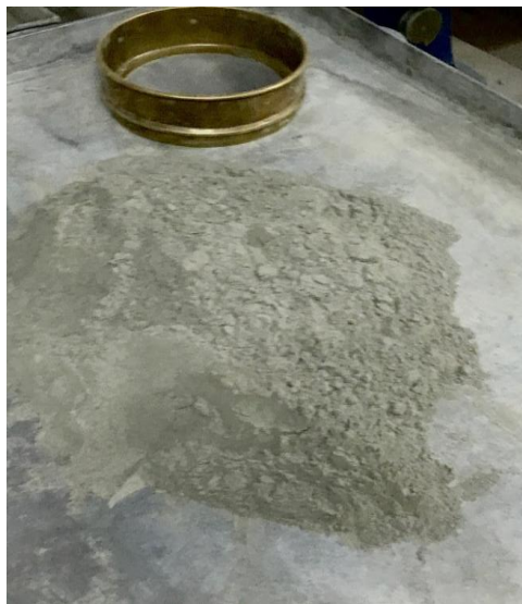
Figure 3.6 fineness test of cement
