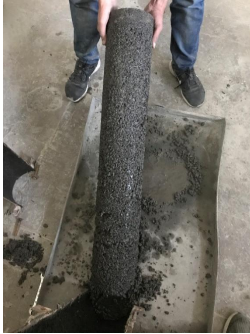
Figure 4.7 (a) de-molding of sample
