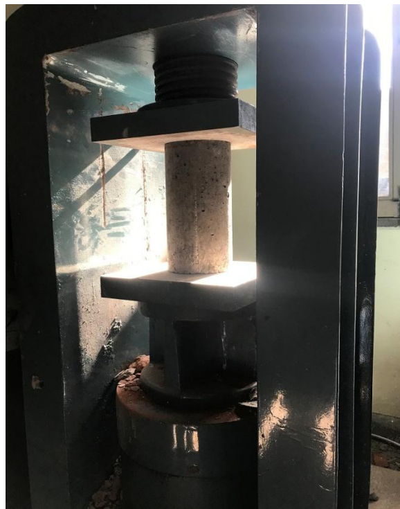
Figure 3.15 Testing under CTM
