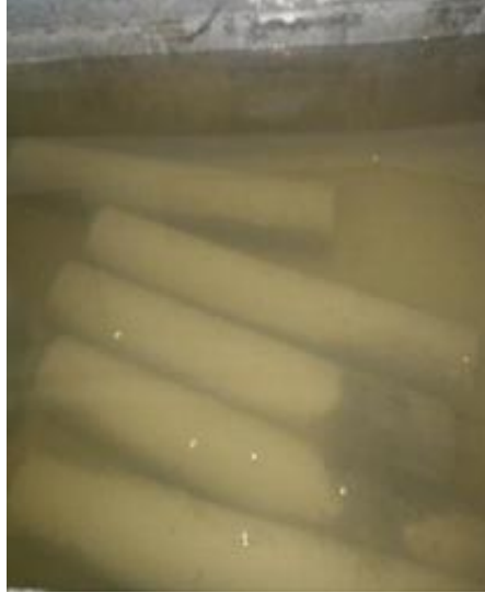
Figure 4.8 curing of sample in curing tank
