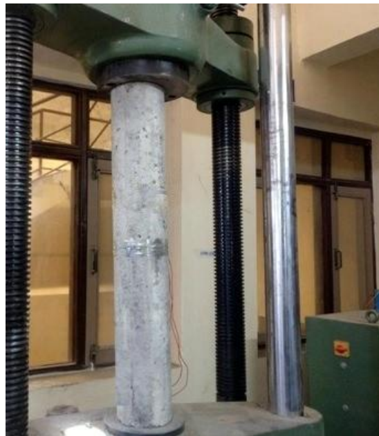
Figure 4.9 Compression testing under UTM
