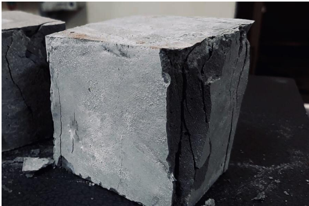
Figure 3.7 Crushed cement specimen
