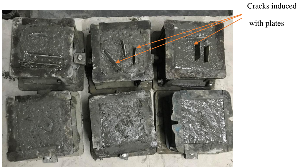
Figure 3.7 Concrete cube specimens with cracks induced (top) and without cracks (bottom)
