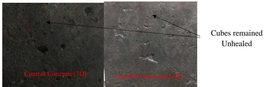
Figure A.4.1. Control concrete sample after 7 and 21 days of concrete cubes curing.
