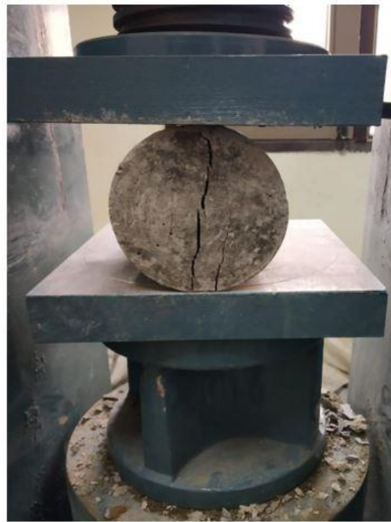
Figure 3.6 Split tensile strength test under CTM
