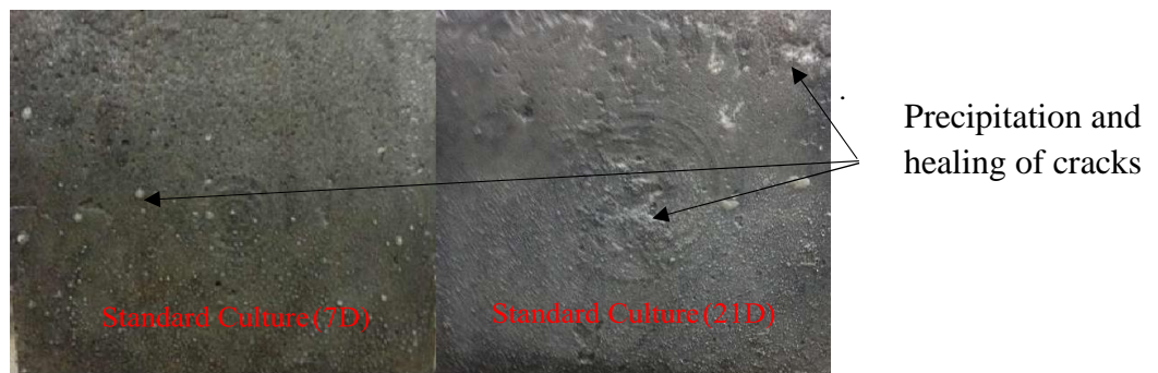
Figure A.4.2. Potential of crack healing by standard culture seen after 7 days and 21 days of concrete cubes curing.
