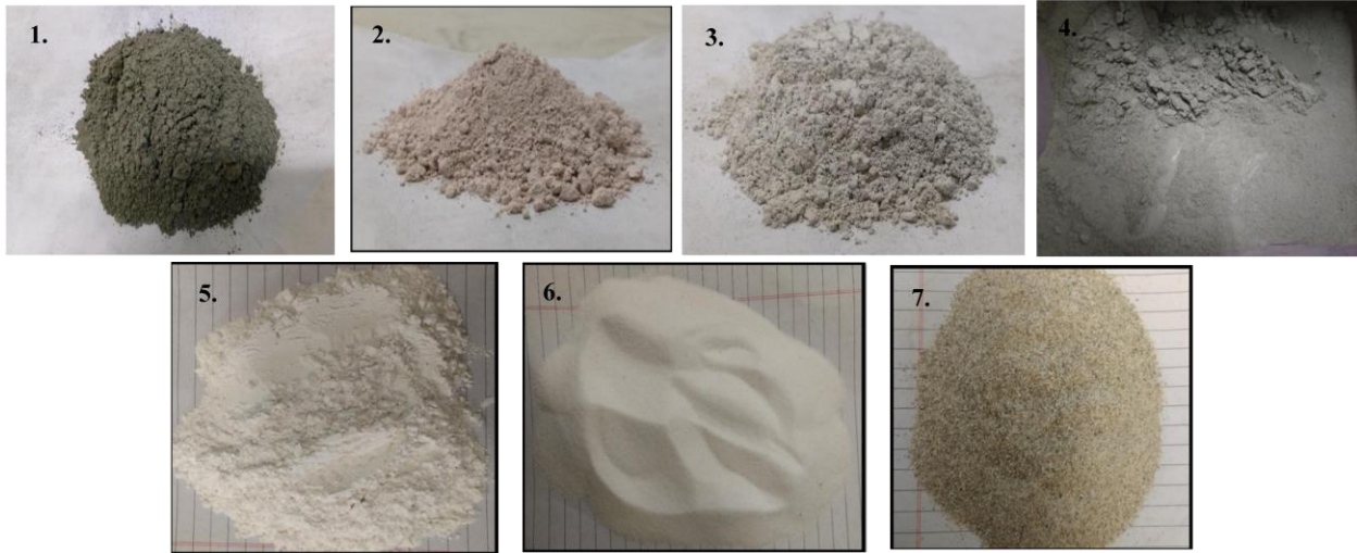
1. Cement 2. Metakaolin 3. Ultra fine Slag 4. Silica fume 5. Quartz Powder 6. Quartz Sand 7. Manufactured Sand.
