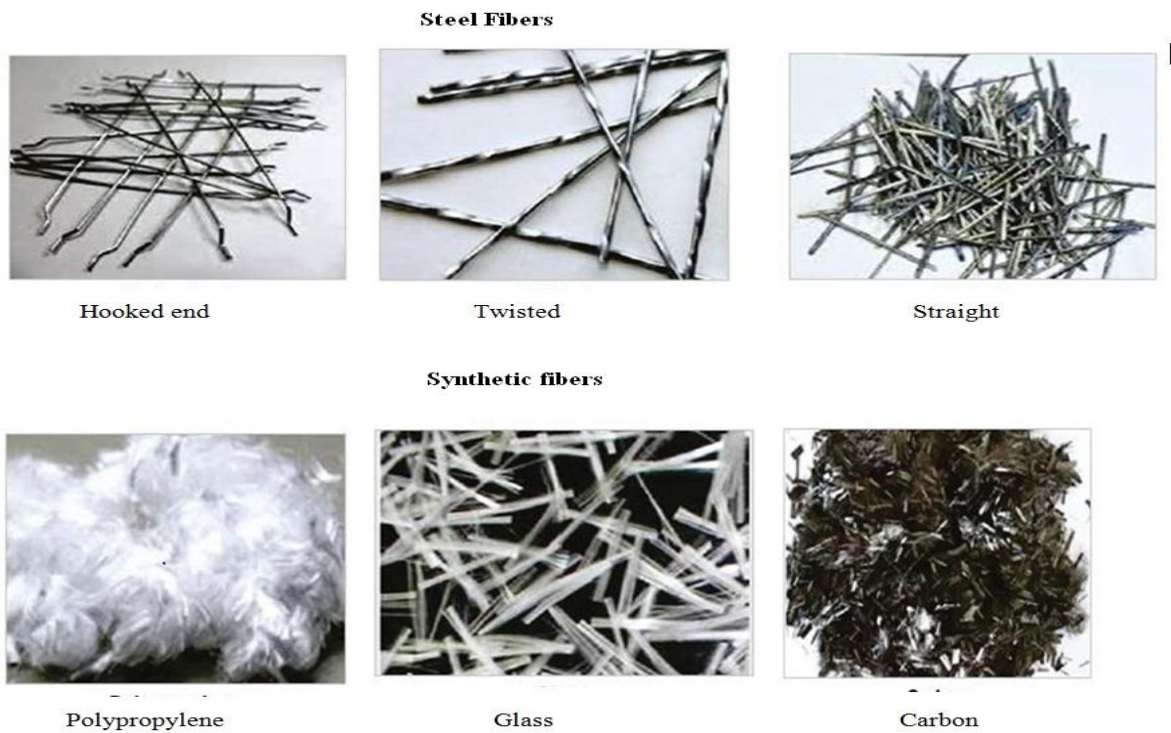
Fig. 1.2. Different type of steel and synthetic fiber [5]
