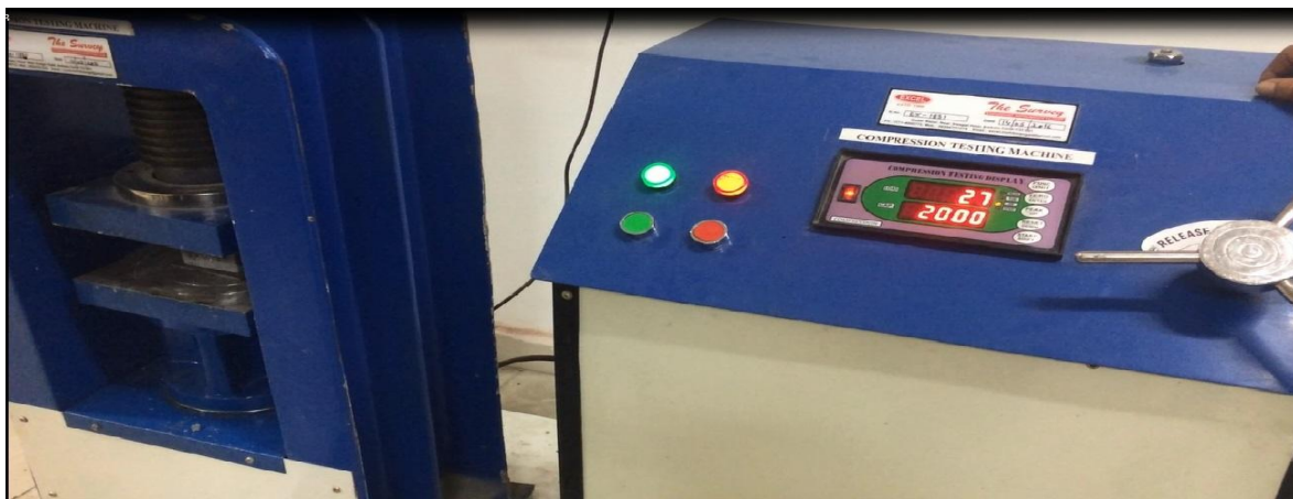
Fig. 4.1 Testing of mortar cube.
