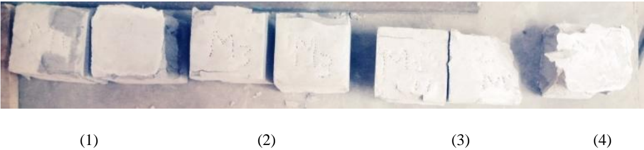
Fig. 5.9 Tested cube samples with fiber and without fiber.
