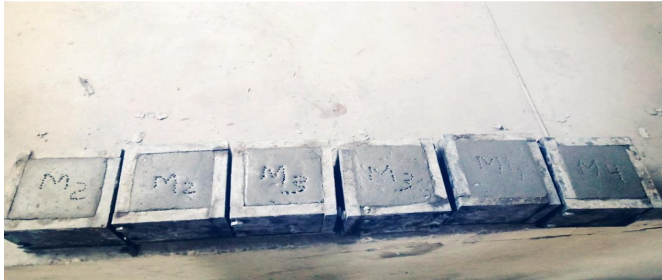
Fig. 3.4. Casted cube samples.
