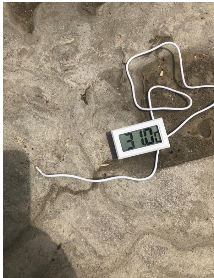
Fig. 4.6 Thermocouple for reading inner pavement temperature
