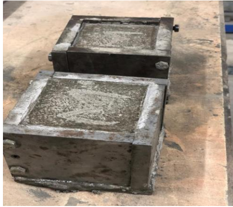
Fig. 4.5 Casting mortar cubes for testing.
