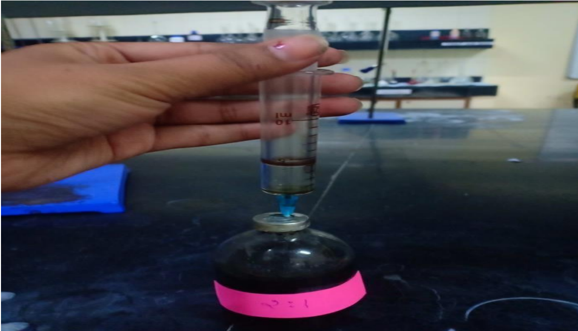
Figure B. 9. Gas Volume Measurement from Serum Bottles Using Glass Syringe
