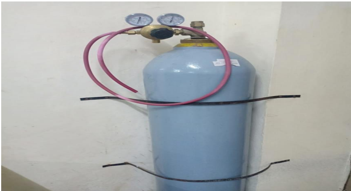
Figure B. 10. Nitrogen Cylinder Used for BMP Test
