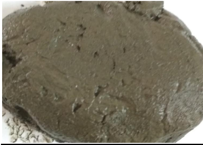
Fig. 3.15 Wet mix at 0.26w/c ratio
