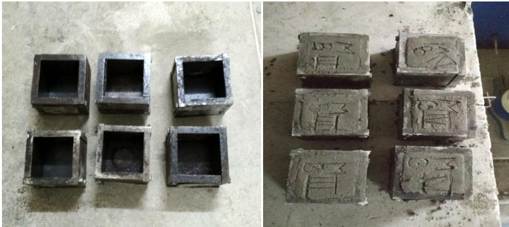
Fig. 3.18 Casting of cube
