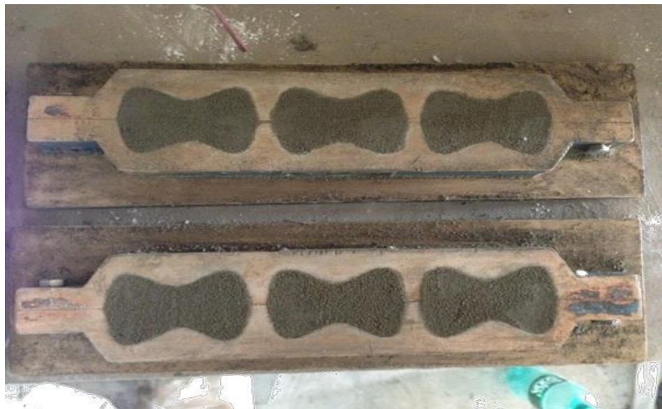
Fig. 3.10 Preparation of briquette specimen
