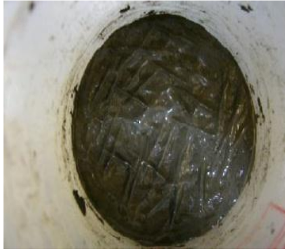
Fig. 3.14 Wet mix at 0.25 w/c ratio
