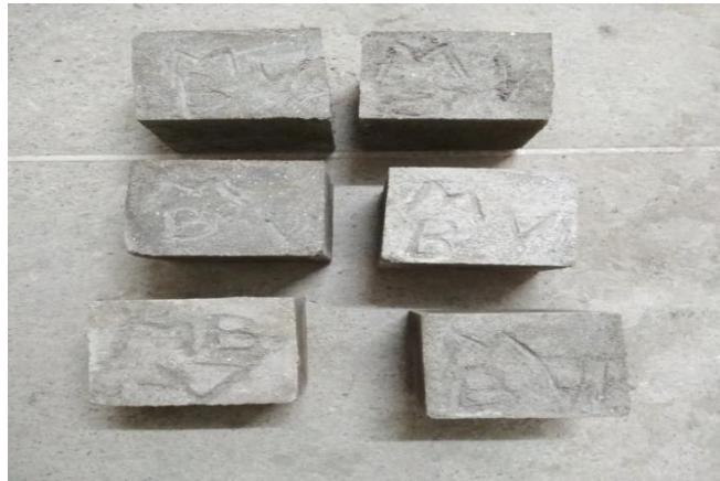
Fig. 3.9 cement mortar casted cube
