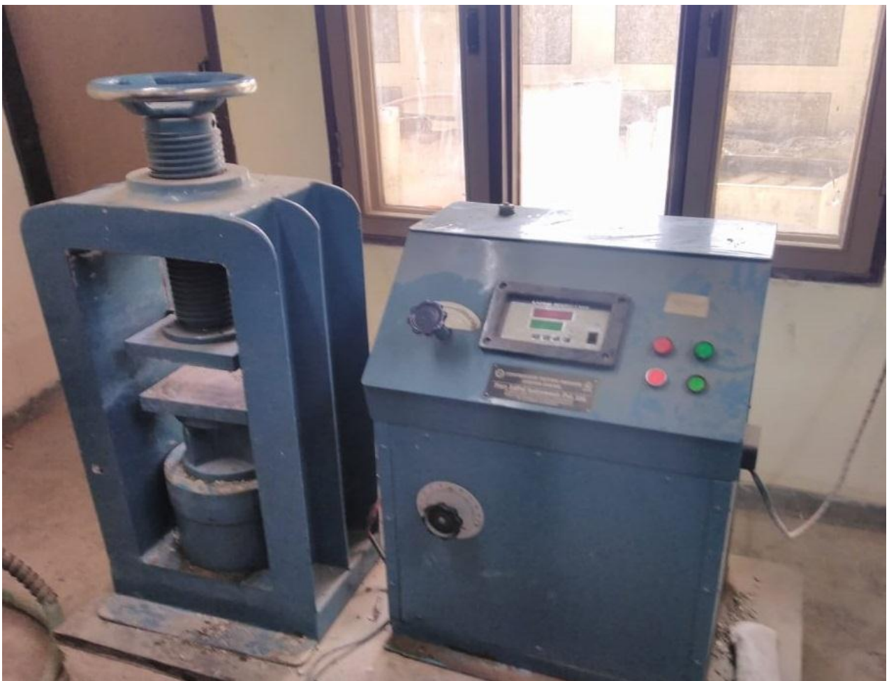
Fig 4.5 Testing of cubes in CTM
