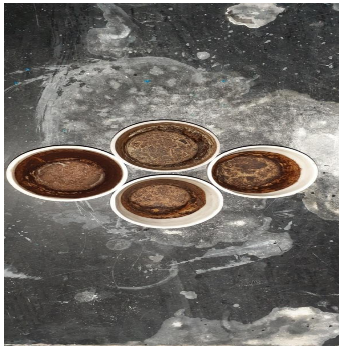
Figure 3.6 Oven dried sample for total solid determination
