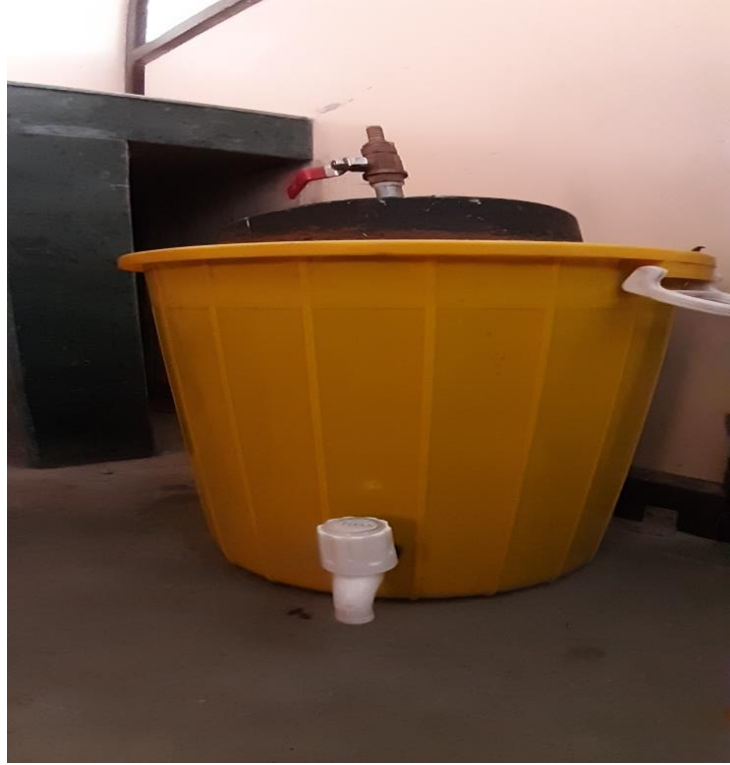
Figure 3.3 Digester 3(50% CD & 50% FW)
