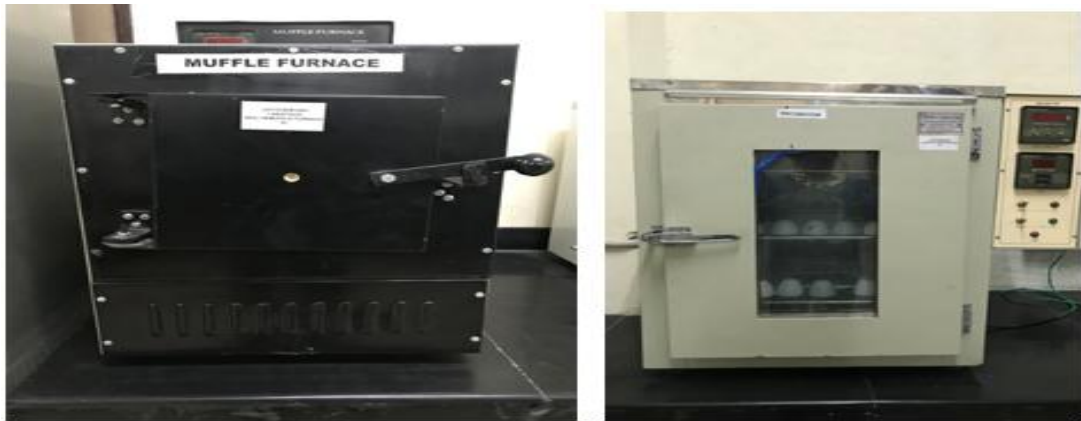
Figure 3.7 Device used in drying sample (a) muffle furnace (b) oven
