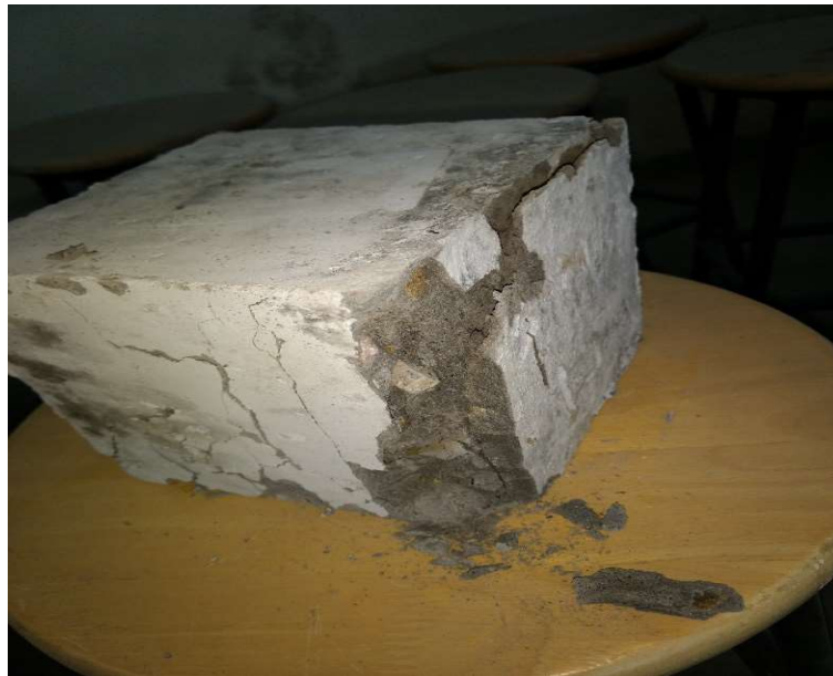
Figure -5 Concrete block after testing
