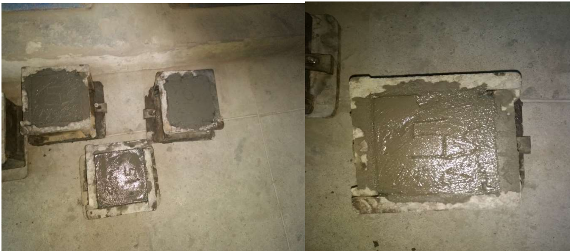
Figure–3 Casting of concrete in mould
