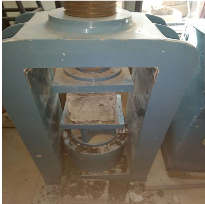
Fig - 7 Compressive strength testing
