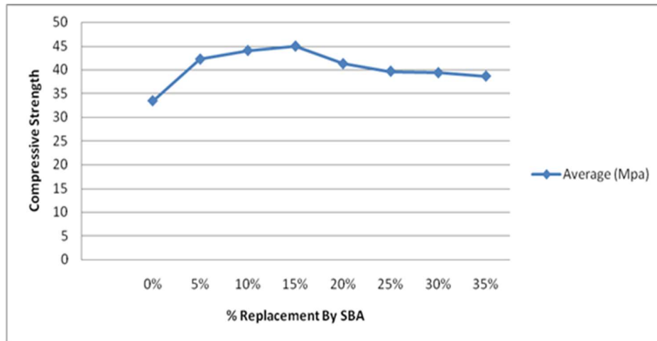
Figure 8: Average Compressive Strength for 7 days using Sugarcane Ash (SBA)
