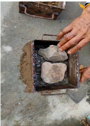
Figure 3.9: Placing of two stones in mould
