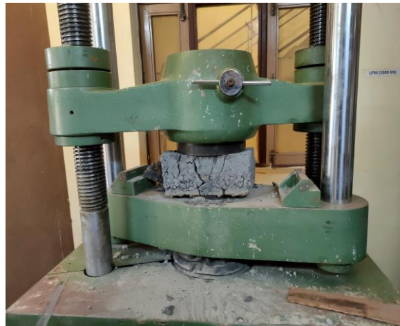
Figure 3.11: Testing of blocks in UTM machine
