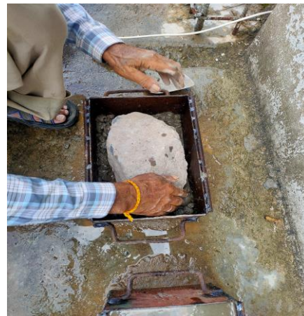
Figure 3.8: Placing stone in Mould
