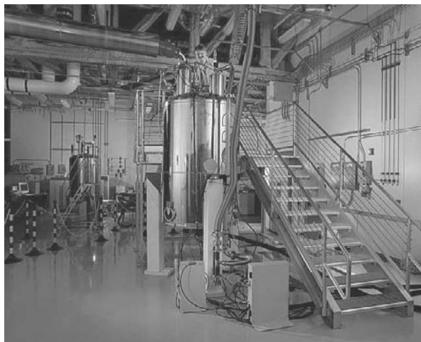
Figure 7.6: An 18.8 T, 800 MHz nuclear magnetic resonance spectrometer at the Pacific Northwest National Laboratory in Kennewick, Washington. A public domain photograph from Wikimedia Commons.
