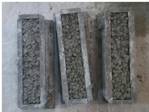
(C) Levelling and finishing of surface of beams
