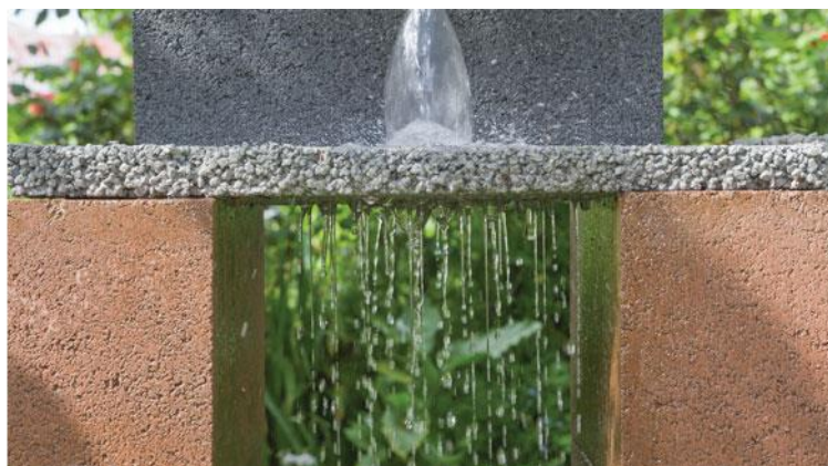
Fig. 1.1.3 Sample of Pervious Concrete
