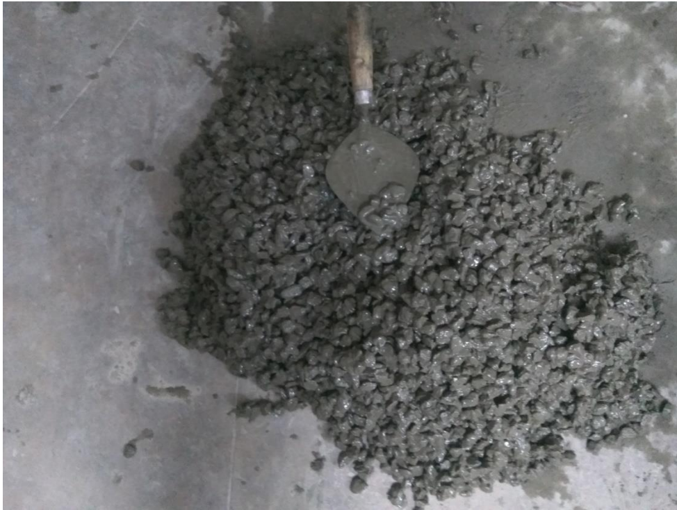
Fig 7.5.3.2: Homogeneous wet mix after adding water
