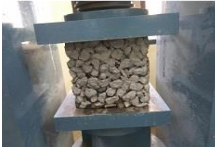
Fig 7.6.2: Placing of cube specimen
