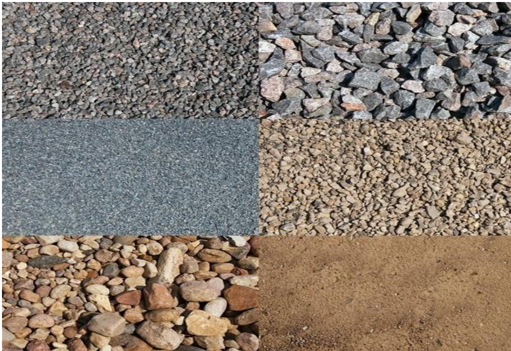
Fig. 1.1.1 Sample of Coarse Aggregate and Fine Aggregate along with Crushed Stone and River Sand
