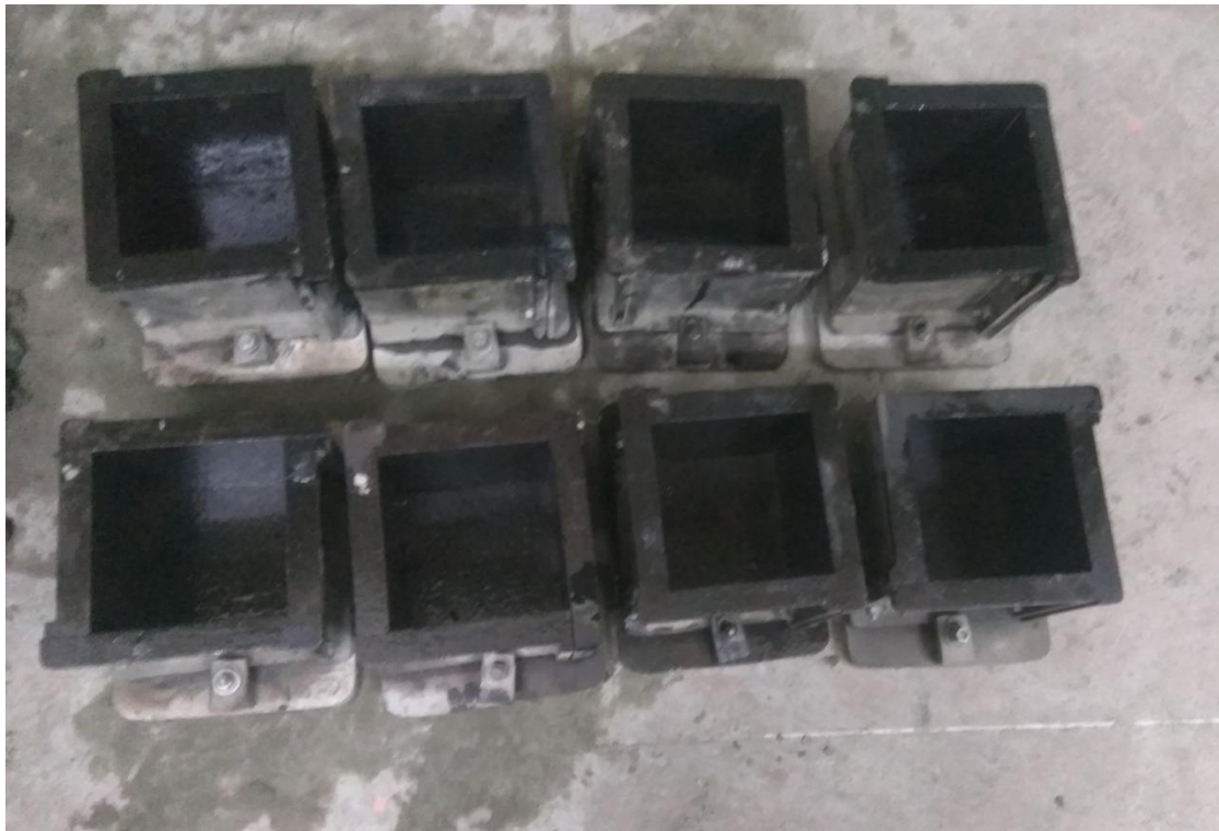
Fig 7.5.2.1: Surface cleaned and Oiled Moulds
