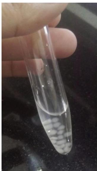
**Fig. 5.** Microcapsules before release of cells in phosphate buffer
