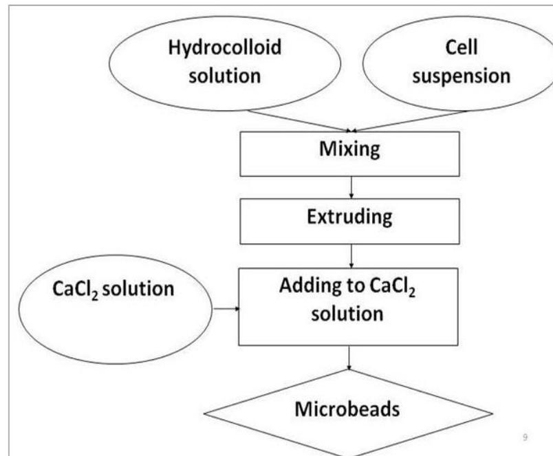
**Fig. 3.** Extrusion Method
