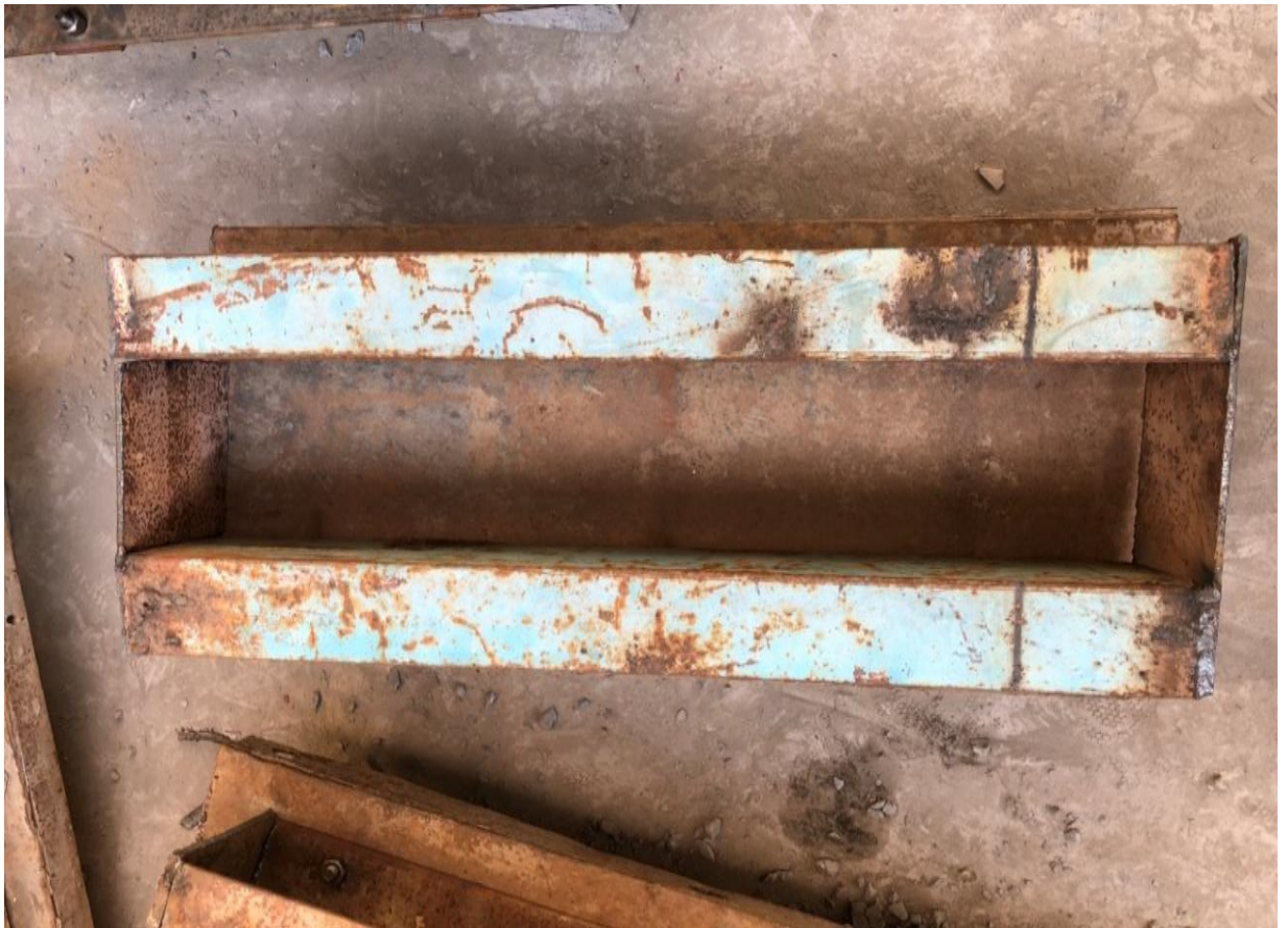
Figure 4.1 Mould of beam
