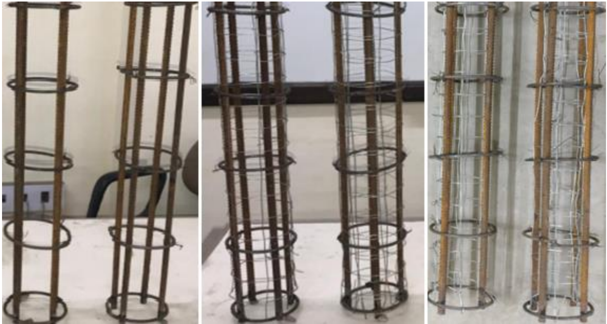
Figure 3.1 Preparation of reinforced cages
