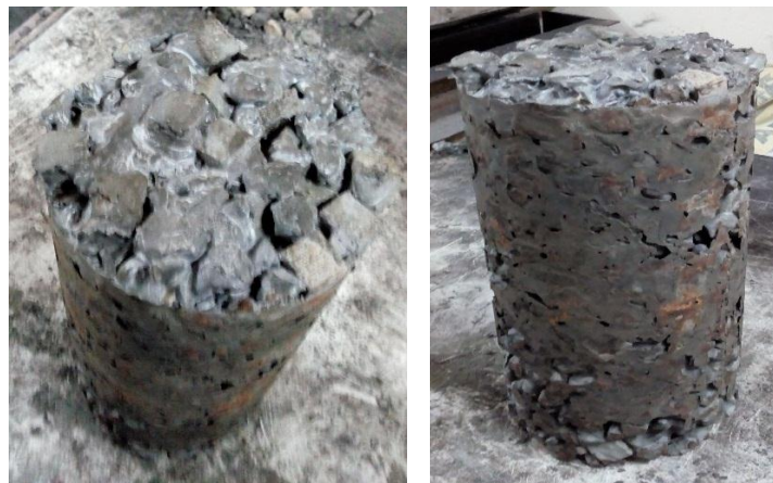
Fig.A7. Prepared samples of porous concrete consisting of 40% replacement
