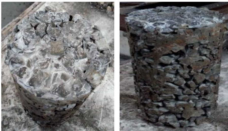
Fig. A4. Prepared samples of porous concrete without any replacement
