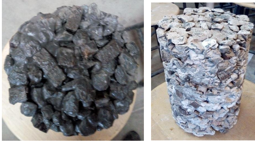
Fig. A6. Prepared samples of porous concrete consisting of 30% replacement
