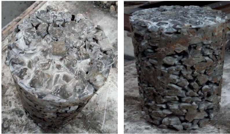
Fig. A5. Prepared samples of porous concrete consisting of 20% replacement
