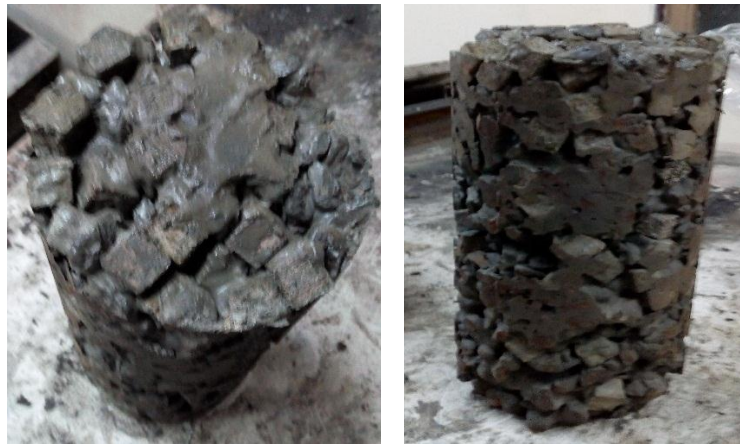
Fig. A8. Prepared samples of porous concrete consisting of 50% replacement
