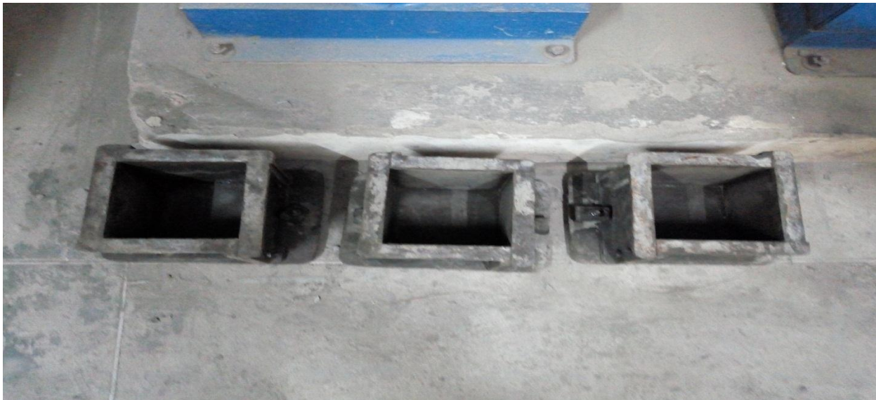
Fig. A2. Cubical Moulds used in the research
