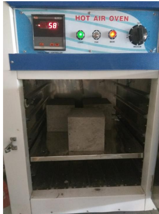
Fig 7.12: Oven dry curing at 75°C
