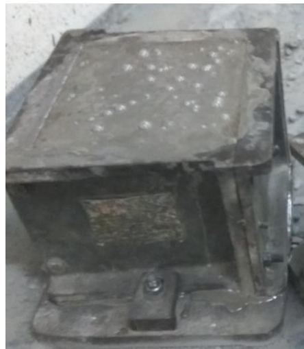
Fig 7.9 Air bubbles travelling to the top of the surface
