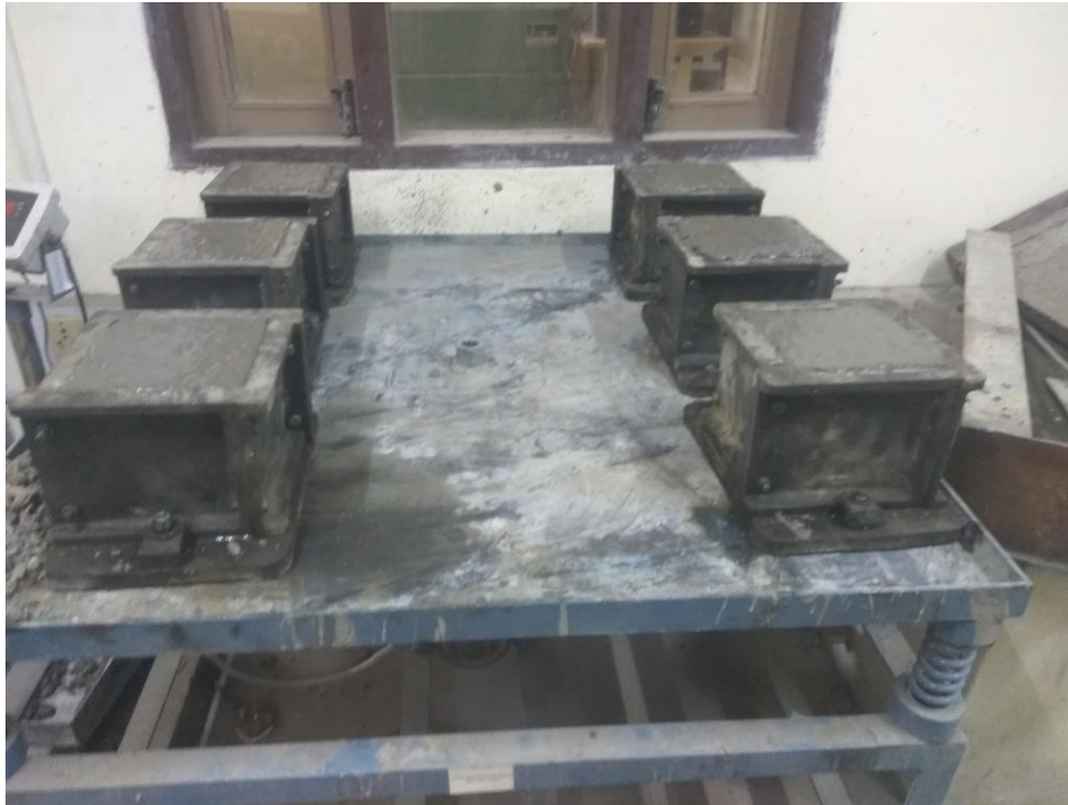
Fig7.8: Table Vibrator to emit out entrapped air
