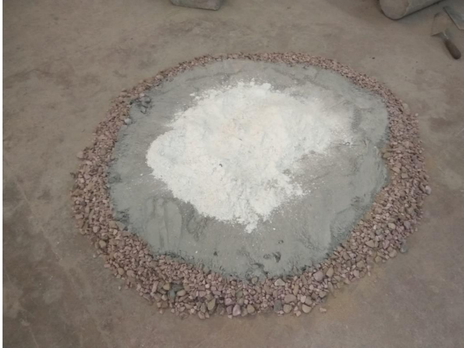
Fig 7.3: Constituents of Geopolymer concrete
