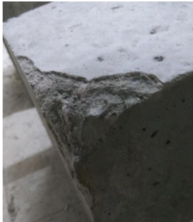
Fig 7.10: Broken edge of cube demoulded without rest period
