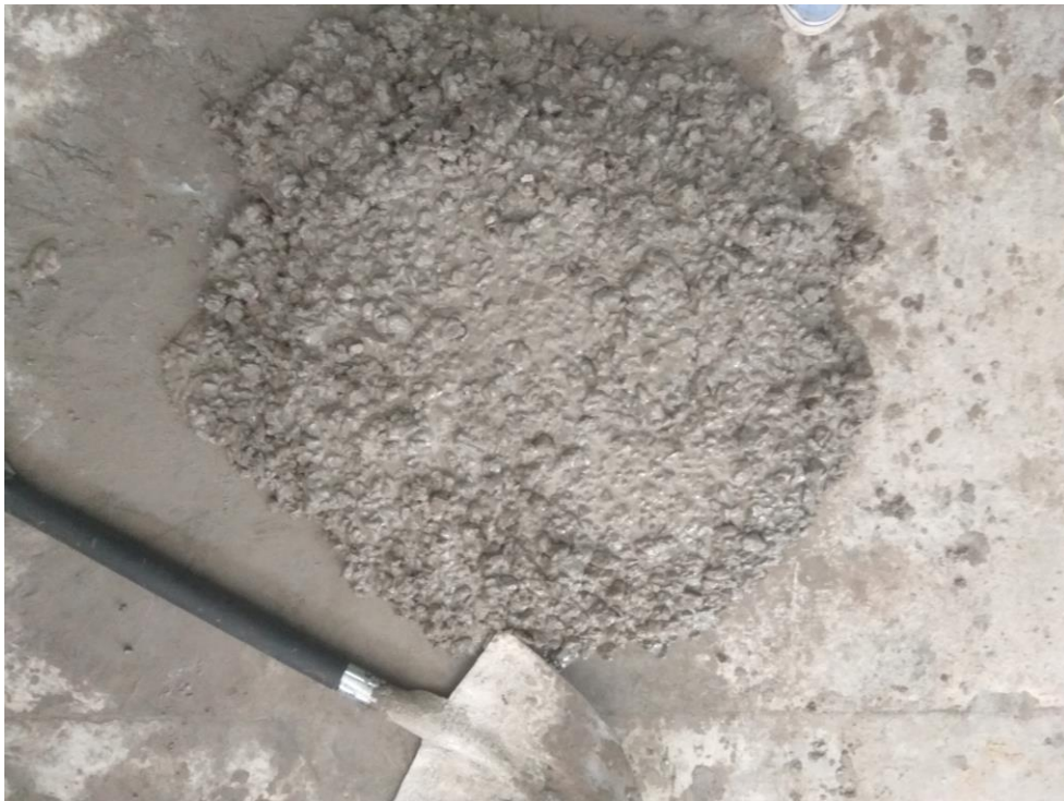
Fig 7.6: Homogeneous Geopolymer Concrete Mix
