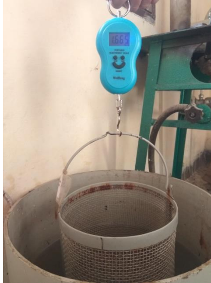
Fig 6.1: Weight of aggregate along with wired basket immersed in water filled bucket
