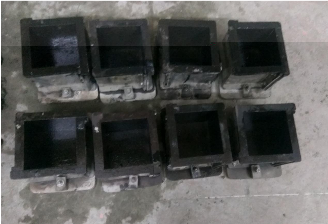
Fig 7.2: Surface cleaned and Oiled Moulds
