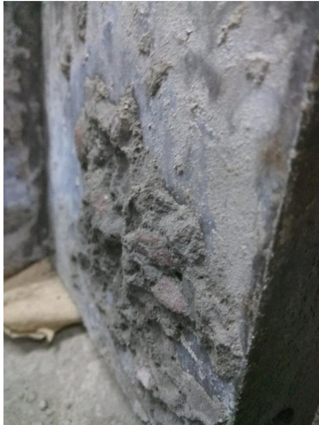
Fig 7.11: GPC without rest period stuck with surface of mould
