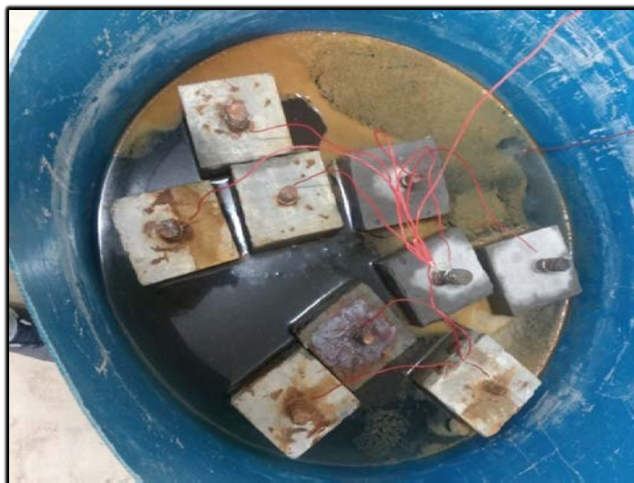
Figure 3.13 Impressed current set up.
