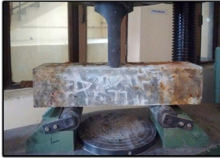
Figure 4.7: Flexure testing of corroded samples
