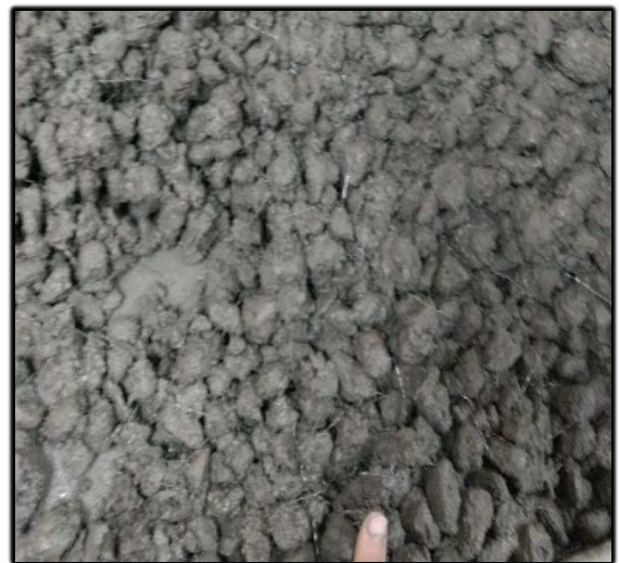
Figure 3.9: Random mixing of steel fiber
