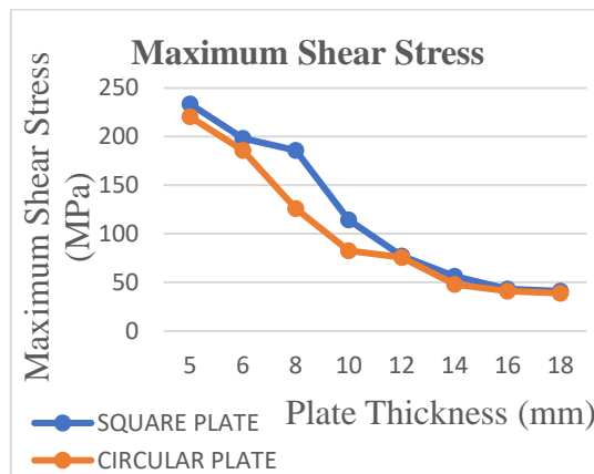
Fig. 4.30: Effect of Plate Geometry on Maximum Shear Stress (Biaxial loading with 8 anchor rods).
