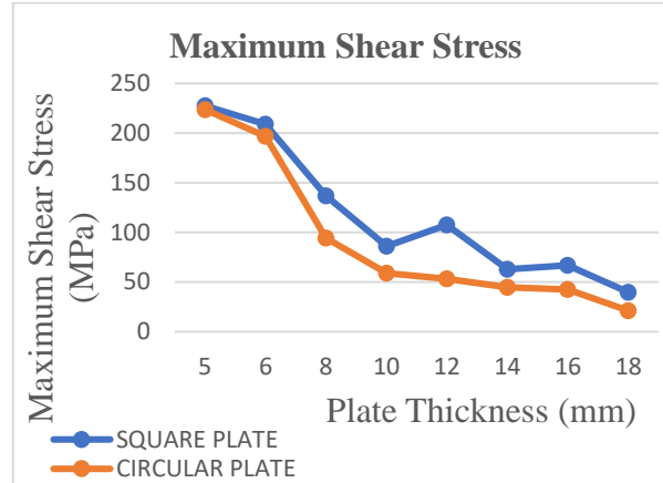
Fig. 4.5: Effect of Plate Geometry on Maximum Shear Stress (Concentric loading with 4 anchor rods).
