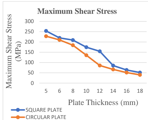
Fig. 4.25: Effect of Plate Geometry on Maximum Shear Stress (Biaxial loading with 4 anchor rods).
