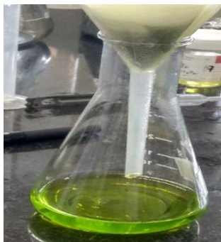
Fig 4.3: MPPCBs e-waste in solution form after performing aqua regia digestion
