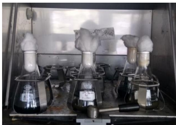
Fig 4.6: Flasks containing bacteria + MPPCBs e-waste kept at incubation at 30°C at 150rpm for 7 days for bioleaching
