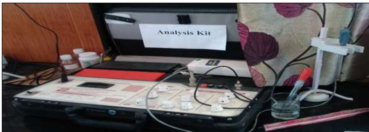
Fig. 3.4 Analysis kit used for determination of pH and Turbidity.
