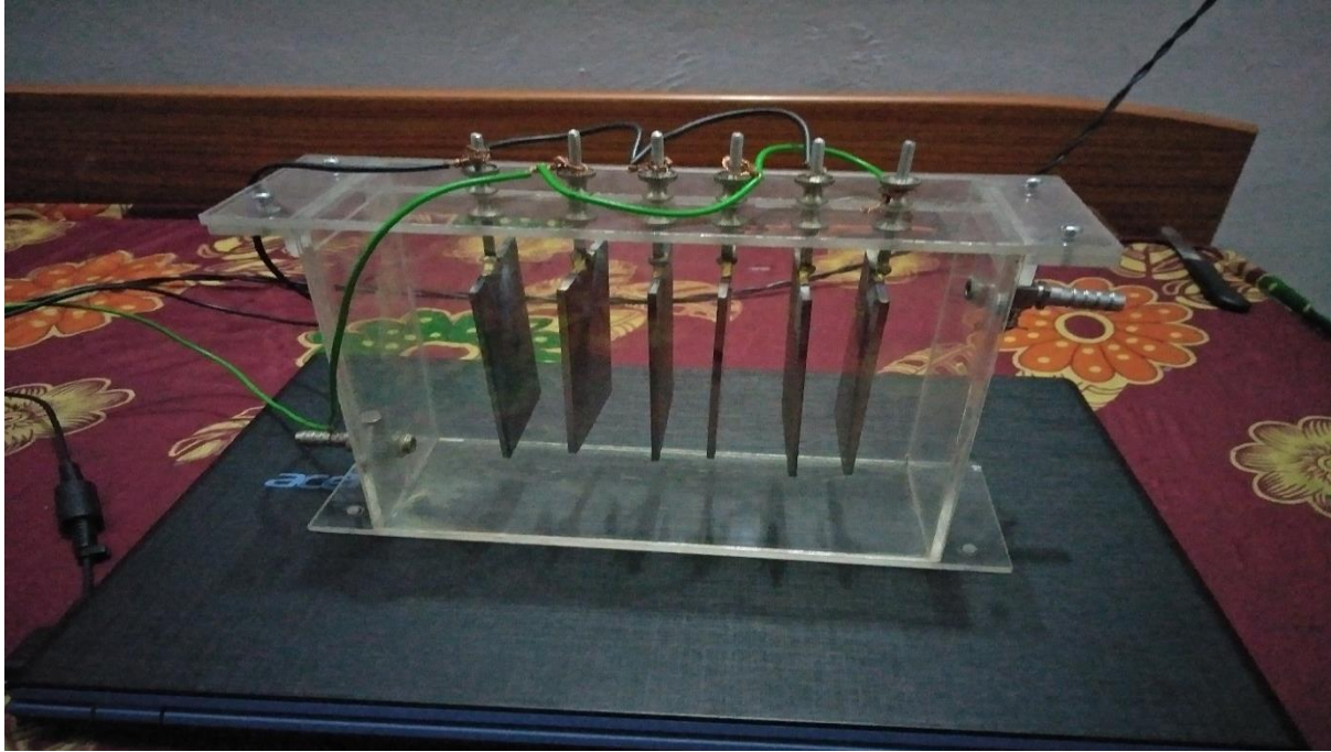
Photograph A.1. Electrocoagulation Reactor
