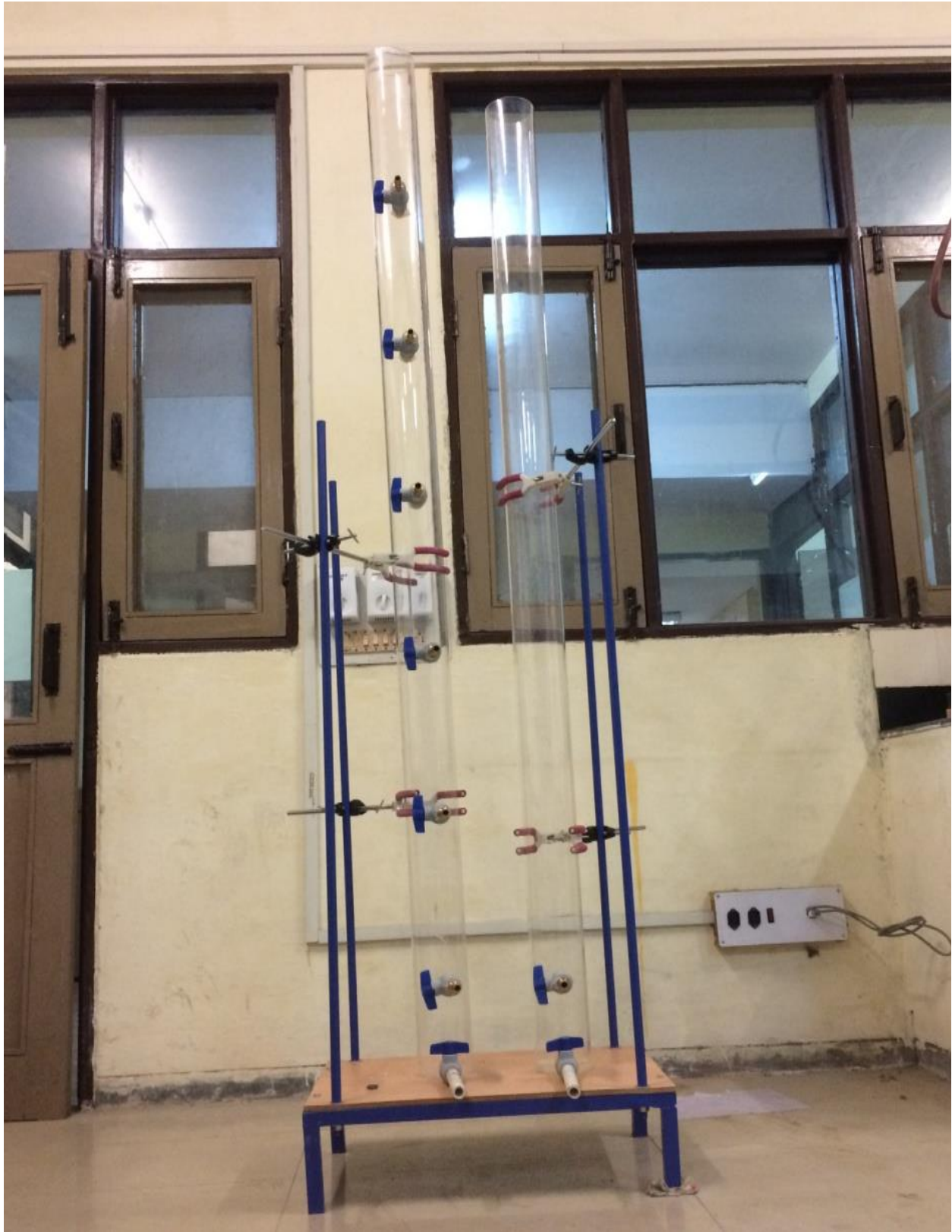
Fig 3.2: Working model of settling columns for laboratory work.
