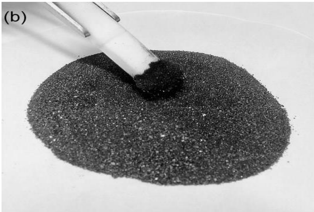
Figure 5 - Photographs of response of (a) bare and (b) \text{Fe}_3\text{O}_4 coated sand particles to magnetic bead.
