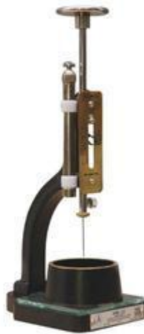
Fig. 3.4 – Vicat's apparatus for initial setting time
