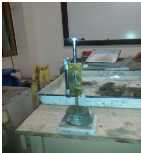
Fig. 3.3 – Vicat’s apparatus for Normal Consistency
