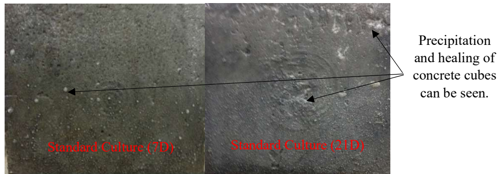
Figure A.4.2. Potential of crack healing by standard culture seen after 7 days and 21 days of concrete cubes curing.
