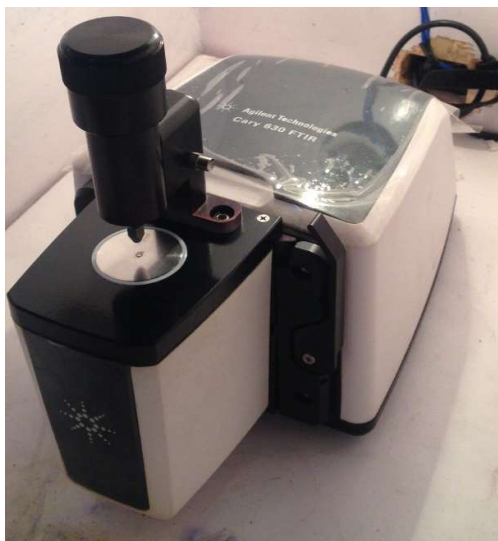
Figure 11. Agilent Technologies Cary 630 FT-IR.
