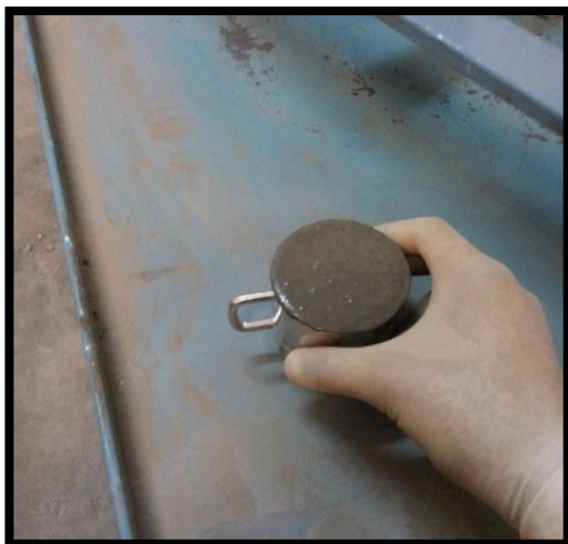
Fig. 3.7: Compacting on vibrating table
