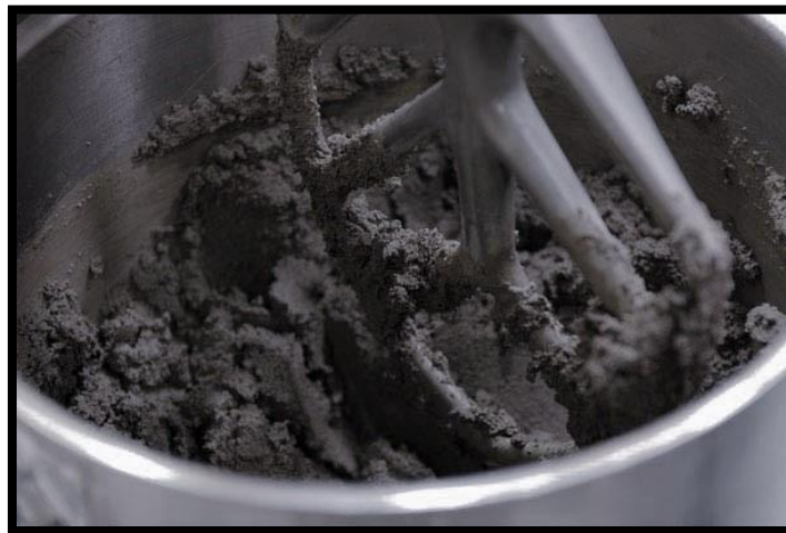
Fig. 3.13: Mixing in Planetarium mixer
