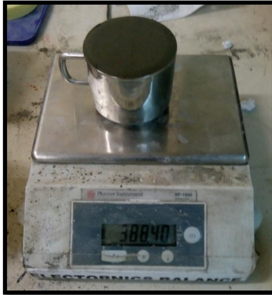
Fig. 3.9: Weighing the compacted paste
