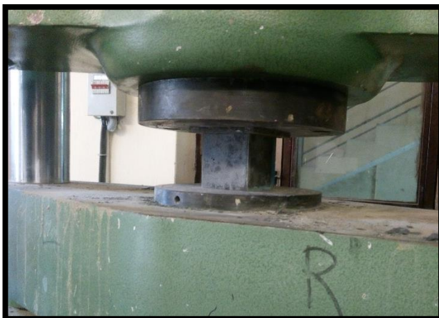
Fig. 3.14: Compression testing in UTM
