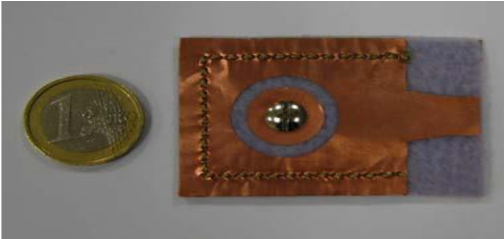
Fig1.7:Wearable antenna, self-adhesive copper tape [Wearable Antennas: Comparison of Different Concepts]
