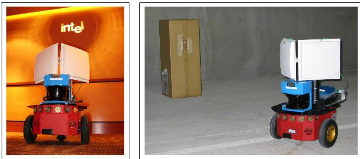
Figure 1.1. Pioneer 2 with Sick Laser Range Finder, RFID reader and two antennas (left).[7]
