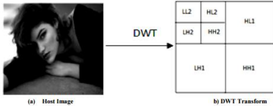
Figure 1.5 Two level DWT decomposition of host image
