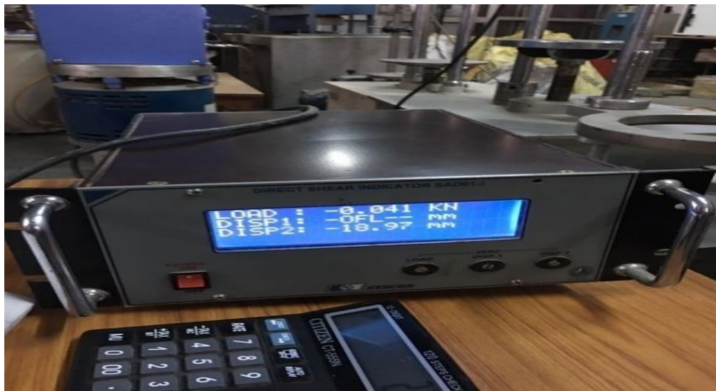
Figure 7(b) – Direct shear apparatus meter displaying load and displacement.
