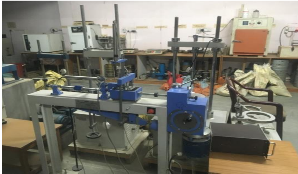
Figure 7(a) – Direct shear test apparatus.
