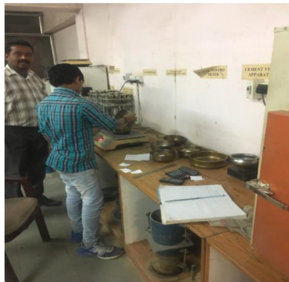
Figure 4(b) – Weight measurement of retained samples in sieve
