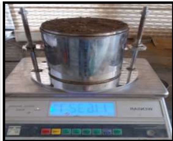
Fig.3. 26 Mould +compacted BS +Base Plate
