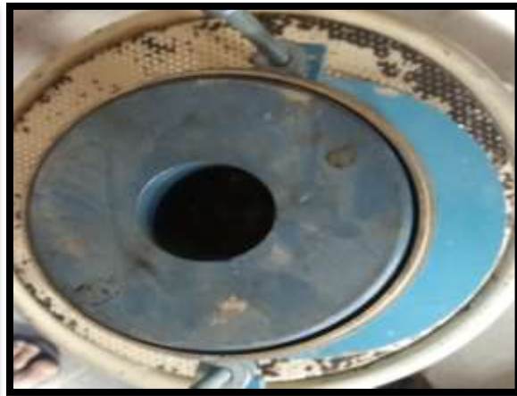
Fig. 3.34 Base plate + Inverted mould with compacted biosolids + Surcharge weight
