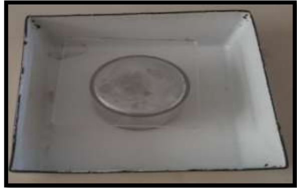
Fig. 3.22 Shrinkage dish fill with mercury
