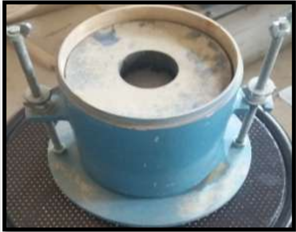
Fig. 3.30 Base plate + Inverted mould with compacted biosolids + Surcharge weight
