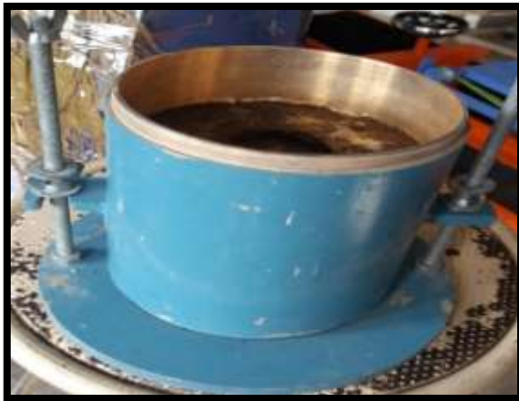
Fig. 3.33 Base plate + Inverted mould with compacted biosolids
