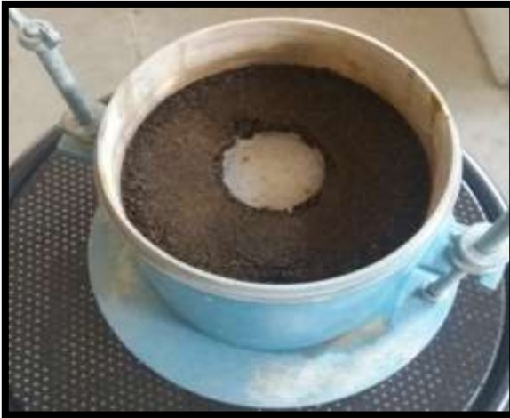
Fig. 3.29 Base plate + Inverted mould with compacted biosolids
