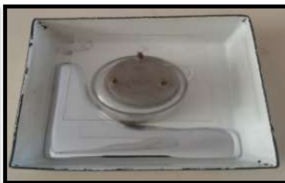
Fig. 3.20 Dry BS pat immersed in glass of full mercury
