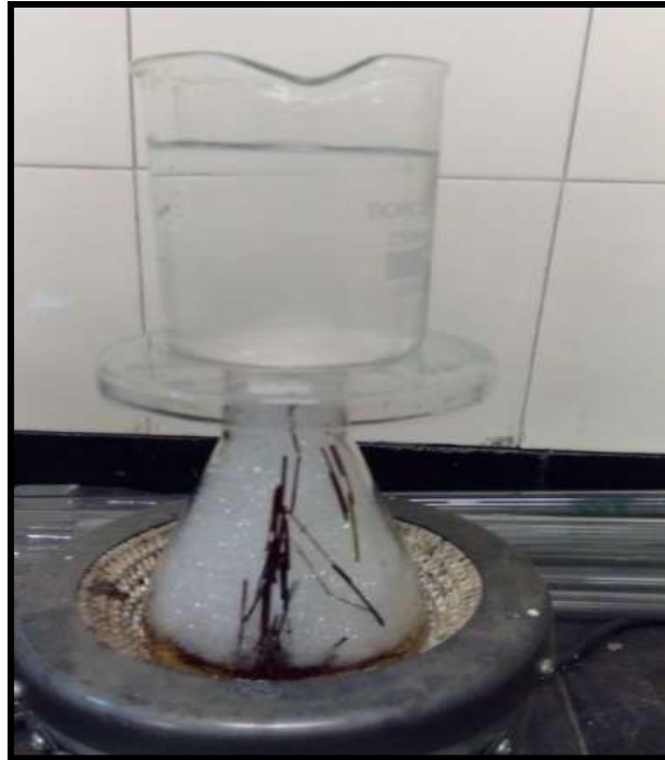
PLATE 3.10 Reflux Procedure during Testing.
