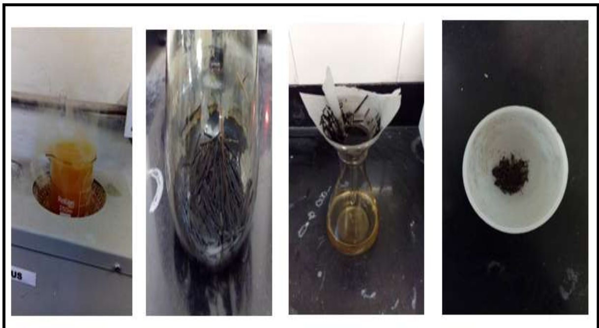
PLATE 3.9 Procedure during Cellulose content test.
