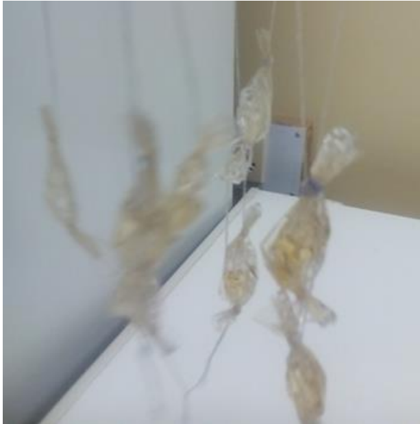
Figure 6: Dialysis in dialysis membrane bag
