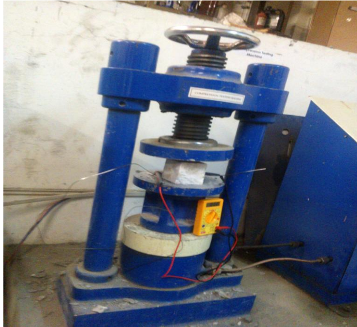
Figure 3.9: Laboratory setup to measure piezoresitivity
