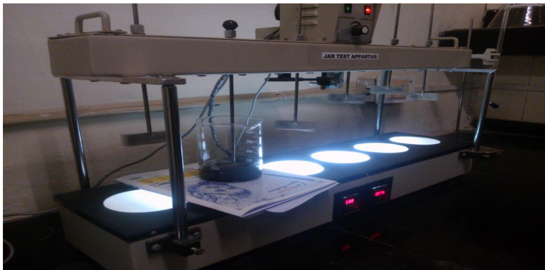
Figure 3.2: Dispersion of CNT with Jar test Apparatus.
