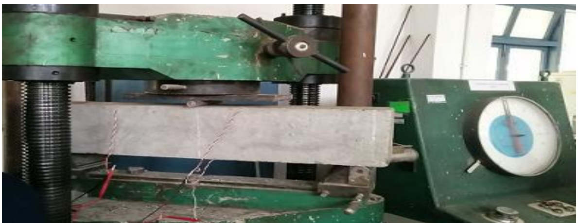
Figure 3.10: Beam testing under UTM
