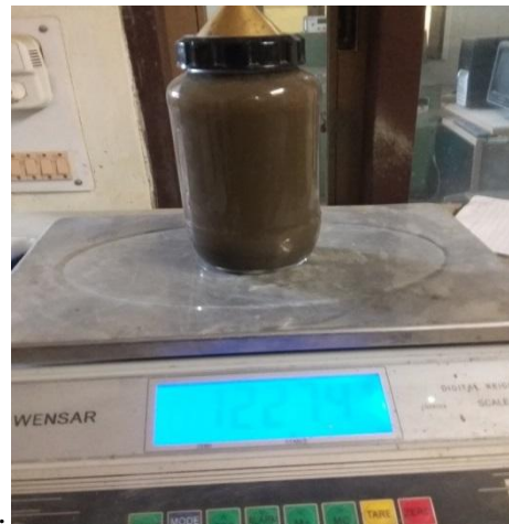
Figure 3.6 Empty pycnometer Figure 3.7 Pycnometer filled with sample
