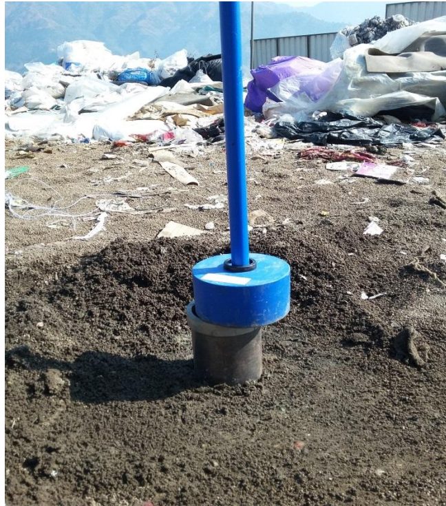
Figure 3.5 In situ core cutter at site
