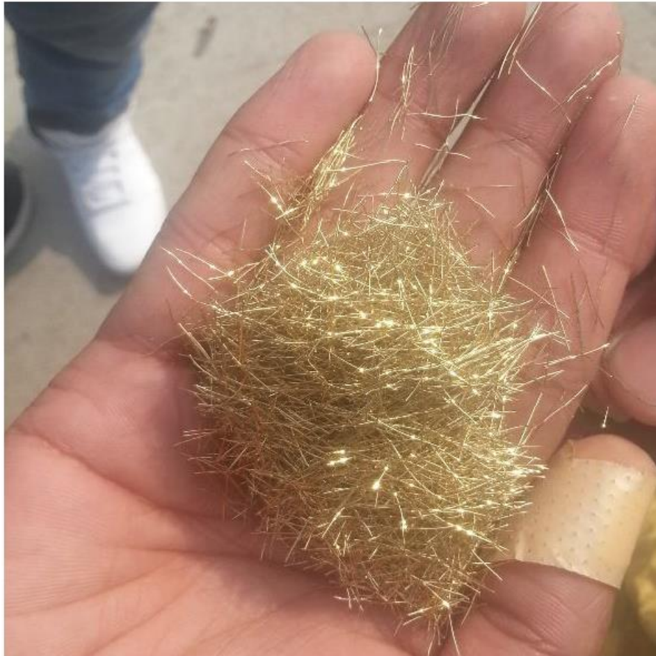
Fig no. 1.4 Brass coated micro steel fibre
