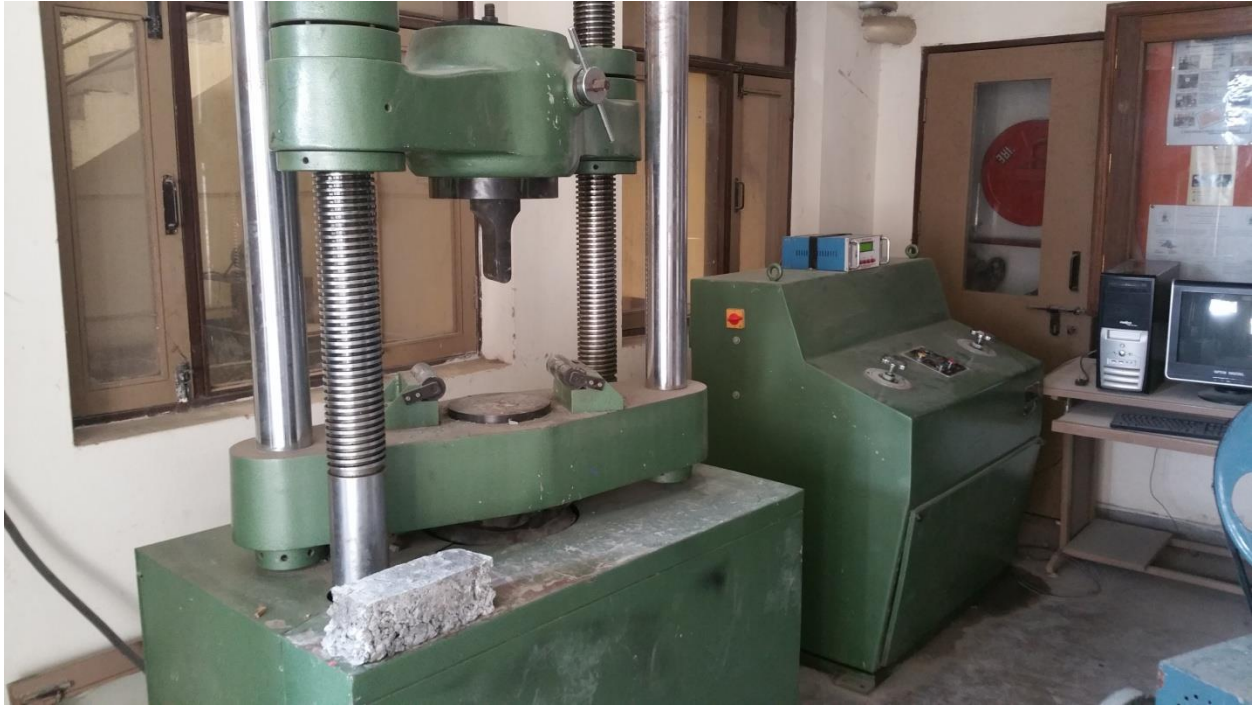
Fig no. 3.8 Flexure testing machine
