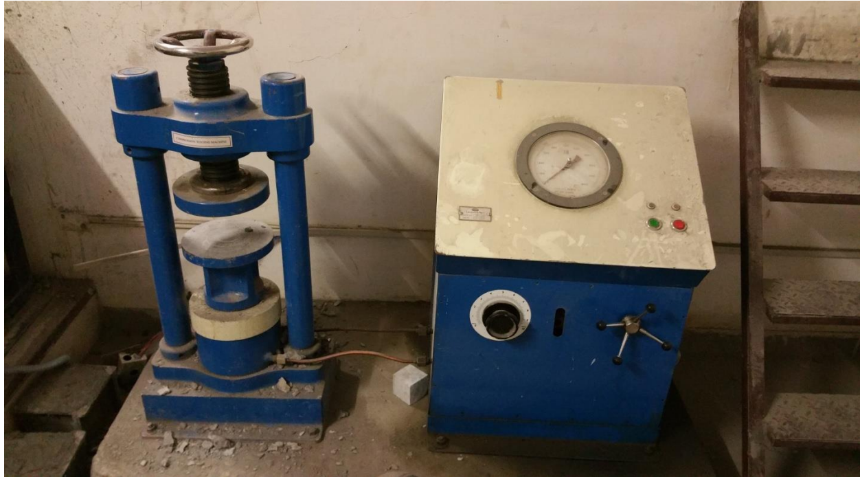
Fig 3.7 Compression testing machine
