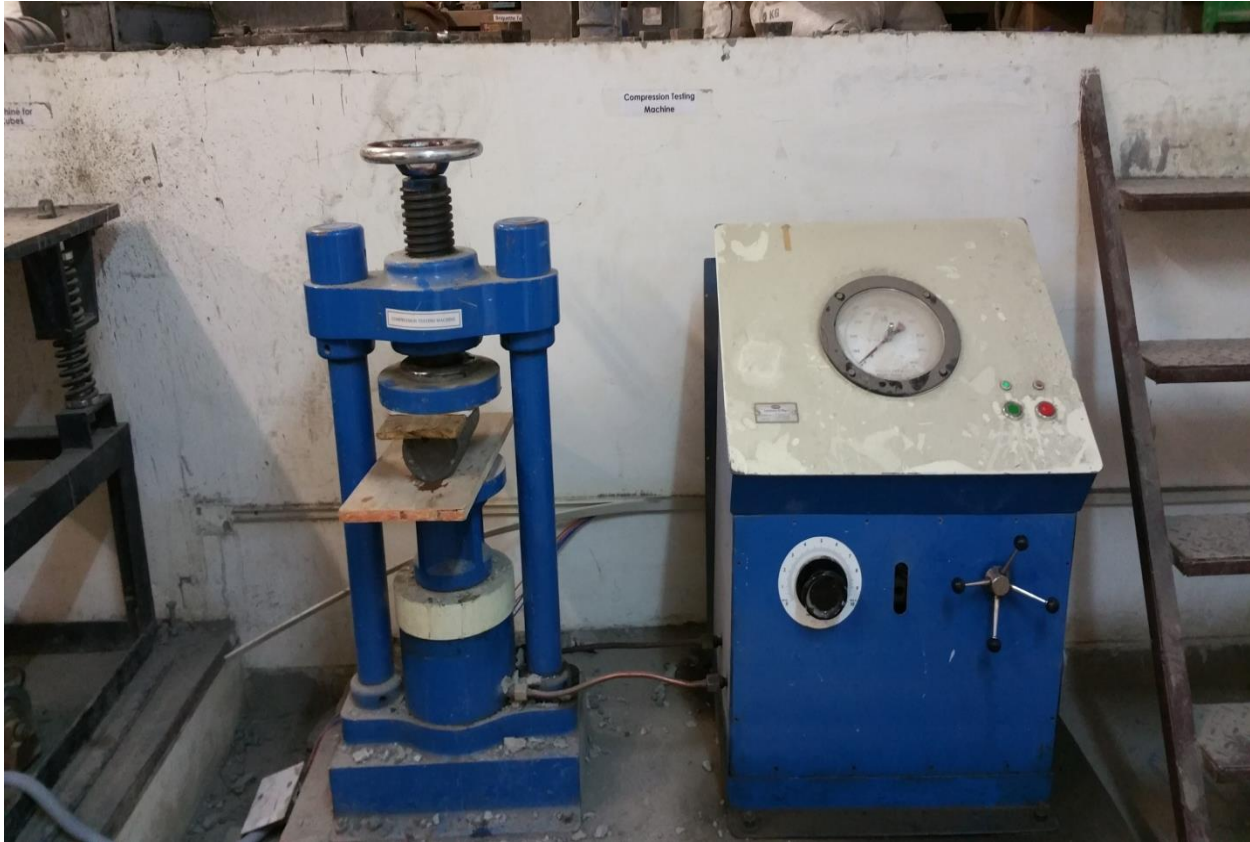
Fig no. 3.9 Split tensile testing machine
