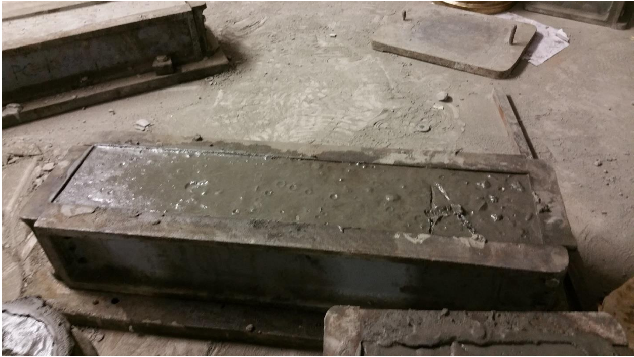
Fig no. 3.6 Casting of specimens
