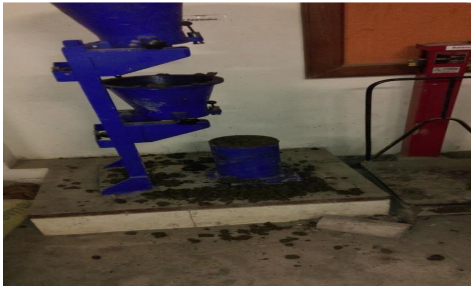
Fig no. 3.4 Compaction testing machine
