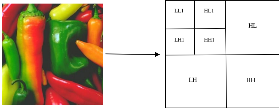
Figure 1.2: Two level DWT decomposition of host image [13-15]
