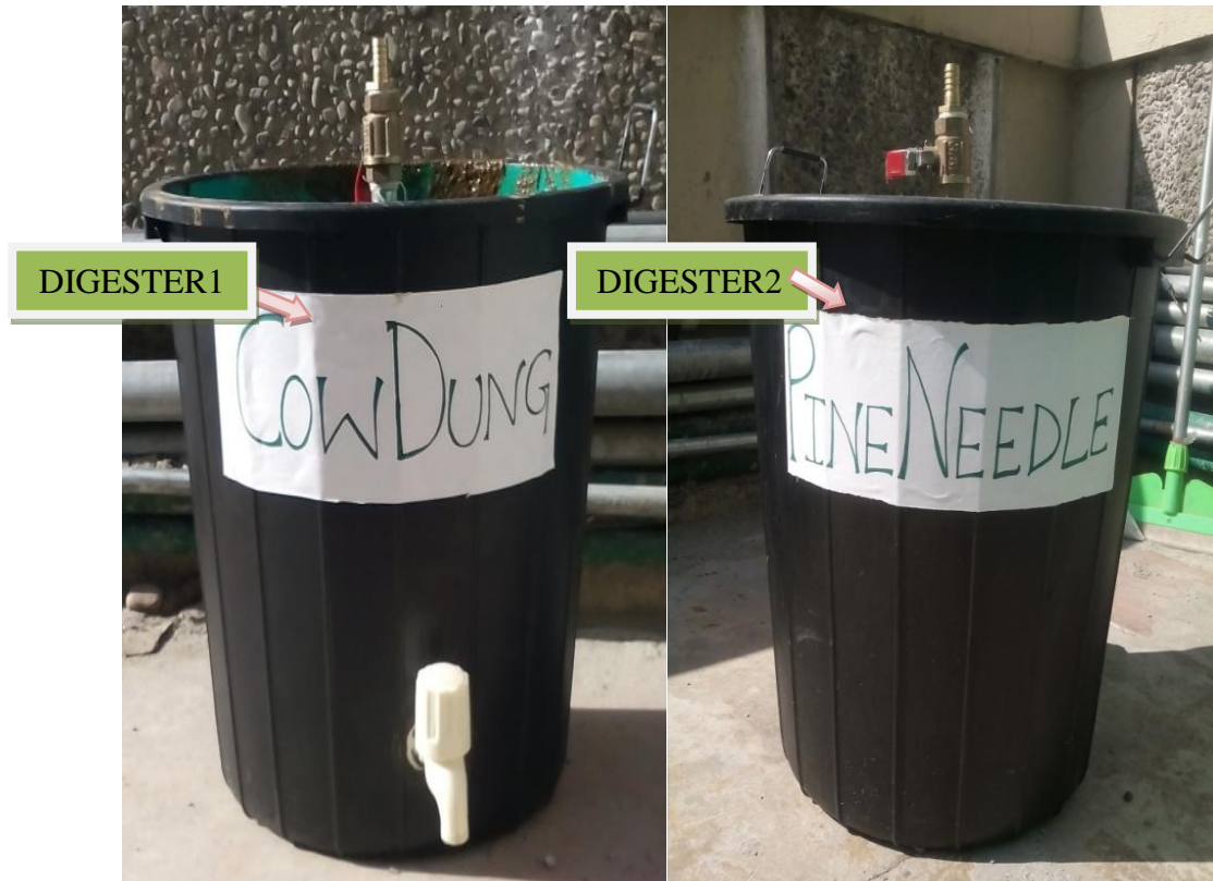
Plate 4.4: Pictorial view of DIGESTER 1 and DIGESTER 2
