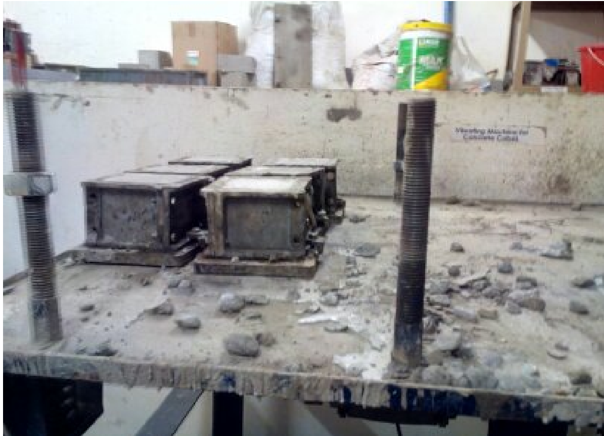
Figure 3.1 Casted Samples for Compressive Strength
