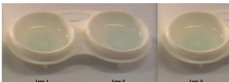
Fig:3.2 Lenses coated with 0.2 % gelatine
