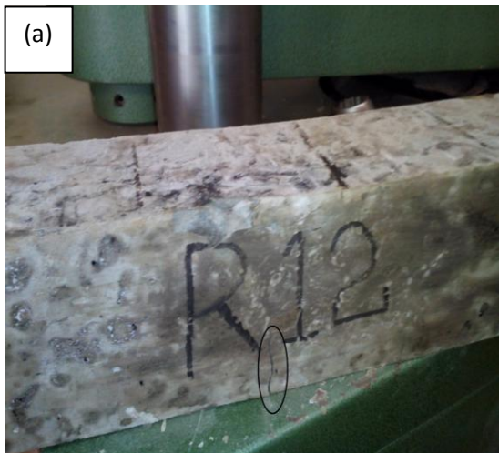
Figure 8 (a,b,c) Plain Concrete Beam placed in U.T.M
