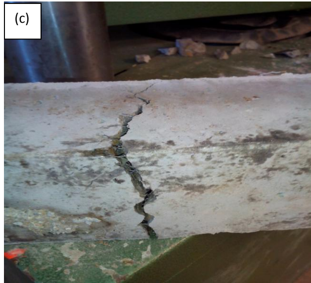
Figure No. 17 (a,b,c) Concrete beams incorporated with steel fibers
