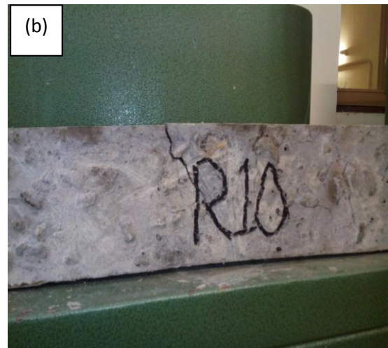
Figure 8 (a,b,c) Plain Concrete Beam placed in U.T.M
