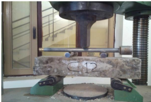
Figure No 03 Plain Concrete Beam placed in U.T.M
