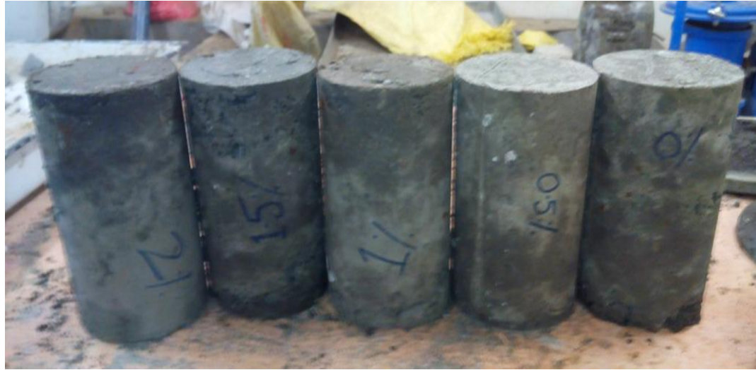
Figure No. 15 Set of cylinders in demoulded state
