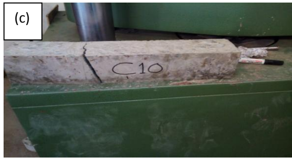
Figure 8 (a,b,c) Plain Concrete Beam placed in U.T.M
